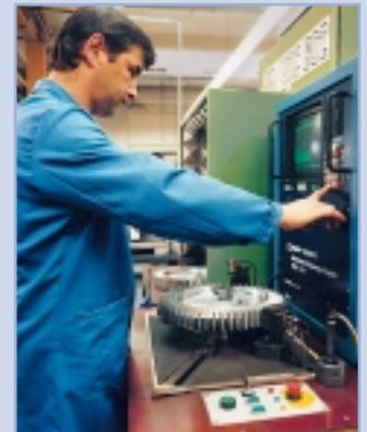
Electronic check of the dimensional accuracy of a G-Series impeller.
