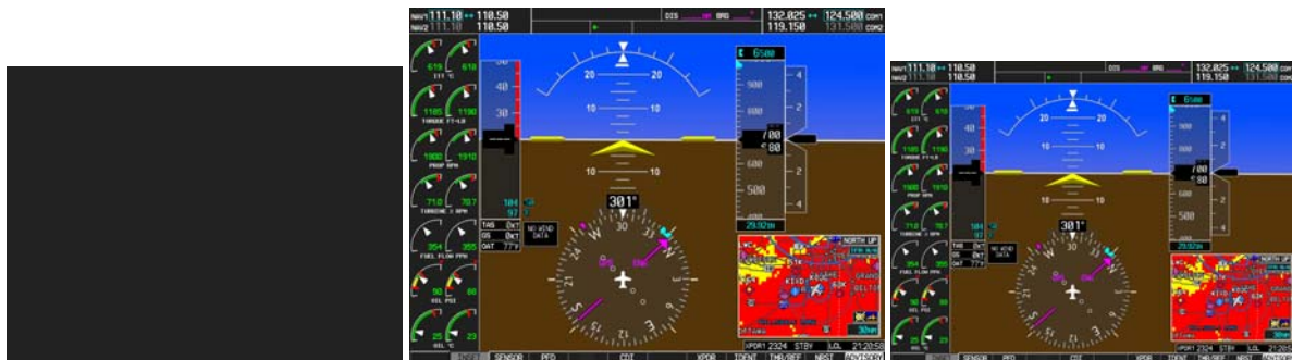
Figure 3-9. Manual Reversion with pilot PFD failure
