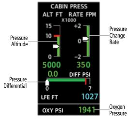
The pressure (in psi) for the oxygen system is shown below the cabin pressurization display under normal display conditions.
