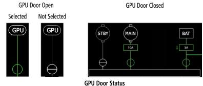
Battery connection status to the main bus is indicated in green; direction of current flow is indicated with an arrow next to the current display. If the battery is disconnected from the main bus, the switch is closed.
