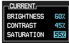
Figure 3-88 External Video Saturation Adjustment
