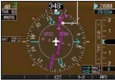
Figure 2-35 Auto-Slewing HSI with Localizer Backcourse Loaded and Shown with the Corresponding Approach Plate
