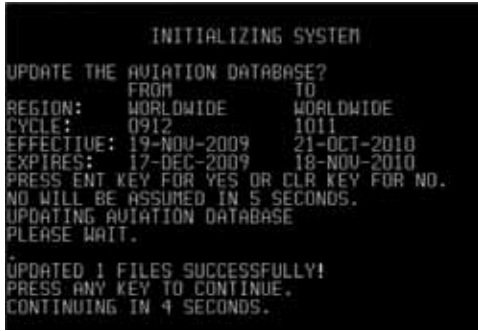
Figure A-2 Database Loading Completed
