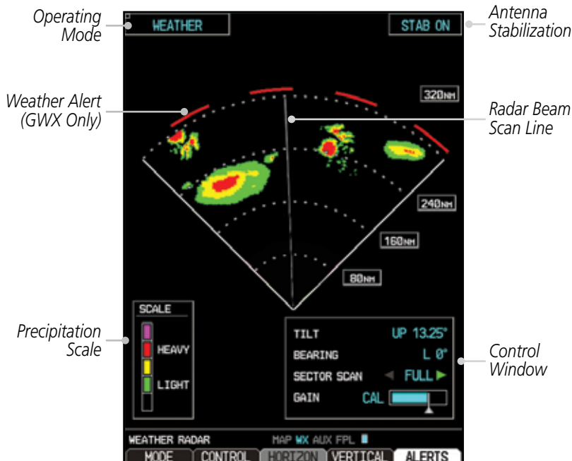
Figure 4-65 Horizontal Scan Display
