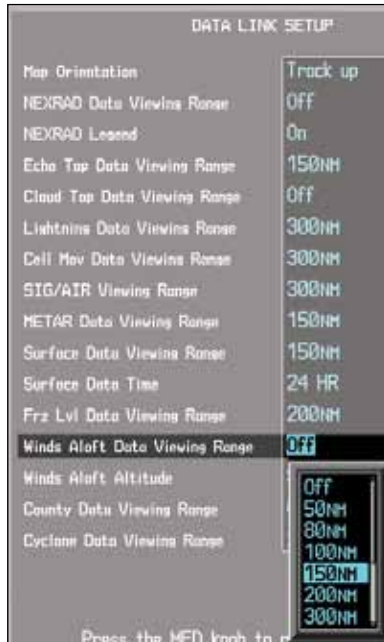
Figure 4-52 Winds Aloft Data Viewing Range Selection
