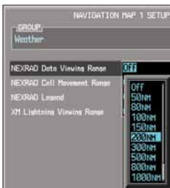
Figure 3-45 NEXRAD Viewing Range Selection
