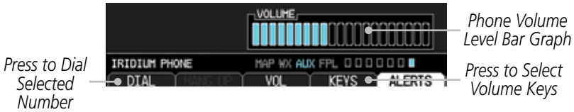
Figure 3-105 Select Soft Keys for Phone Volume Adjustment
