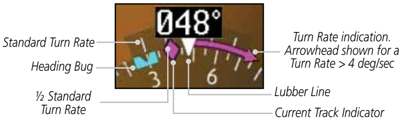
Figure 2-28 Turn Rate Indicator and Trend Vector
