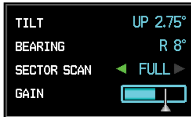
Figure 4-71 Adjust Gain Cal Value
