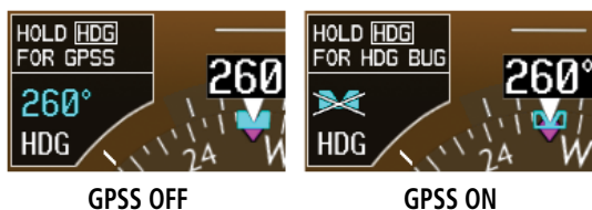
Figure 5-31 GPSS mode control with the HDG key
