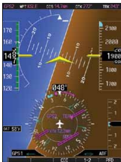
Figure 2-19 Extreme Roll Indication with Display Declutter
