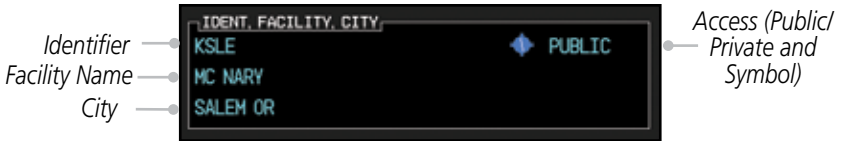
Figure 3-119 Flight Plan Ident/Facility/City Detail
