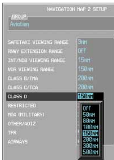
Figure 3-58 Navigation Map Class D Viewing Range Selection
