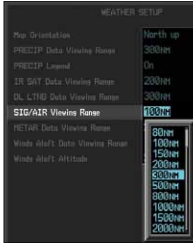
Figure 4-104 GFDS SIG/AIR Viewing Range Selection
