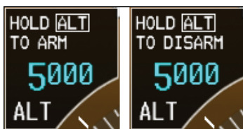
Figure 5-29 Pressing and Holding the ALT Key to Arm/Disarm the Selected Altitude
