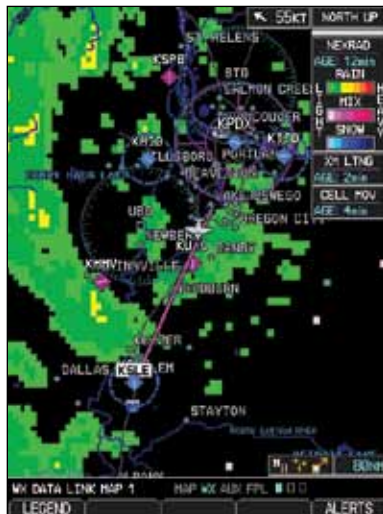
Figure 4-24 XM Weather - NEXRAD
