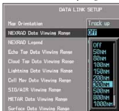
Figure 4-27 NEXRAD Viewing Range Selection
