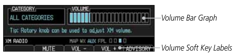
Figure 5-24 XM Radio Volume Controls
