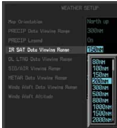
Figure 4-99 GFDS IR SAT Viewing Range Selection
