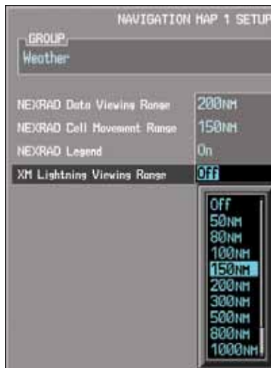
Figure 3-48 Lightning Viewing Range Selection
