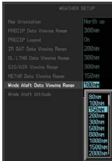
Figure 4-109 Winds Aloft Data Viewing Range Selection
