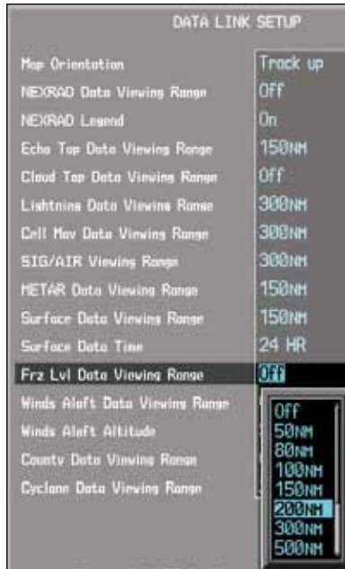
Figure 4-49 Freezing Level Viewing Range Selection
