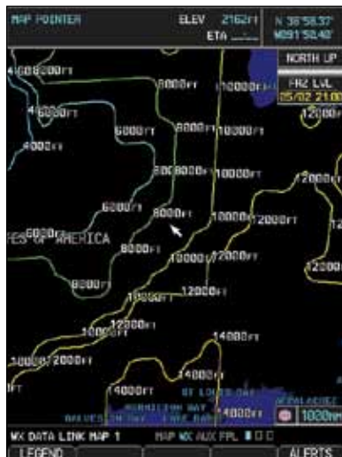
Figure 4-48 XM Weather - Freezing Levels
