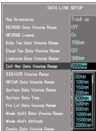
Figure 4-36 Cell Movement Viewing Range Selection
