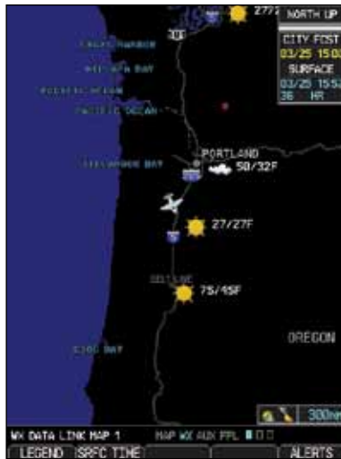
Figure 4-41 XM Weather - Surface Analysis and City Forecast
