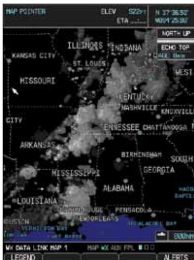
Figure 4-29 XM Weather - Echo Tops
