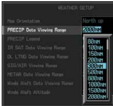
Figure 4-96 GFDS PRECIP Viewing Range Selection
