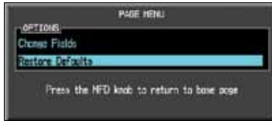
Figure 3-112 Active Flight Plan Page Menu Option Selection to Restore Defaults
