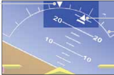
Figure 2-15 Attitude Indicator with a Sky Pointer configuration in a left turn
