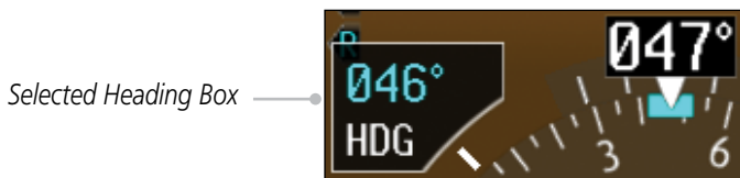
Figure 5-28 Adjusting the Heading Bug
