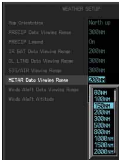
Figure 4-106 METAR Viewing Range Selection
