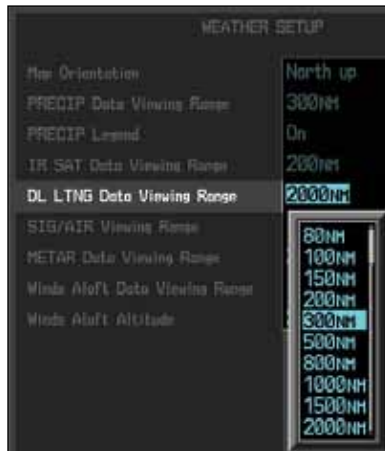
Figure 4-101 GFDS Lightning Viewing Range Selection
