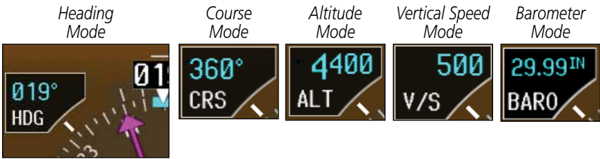
Figure 1-16 Selection Modes Adjusted with the PFD Knob
