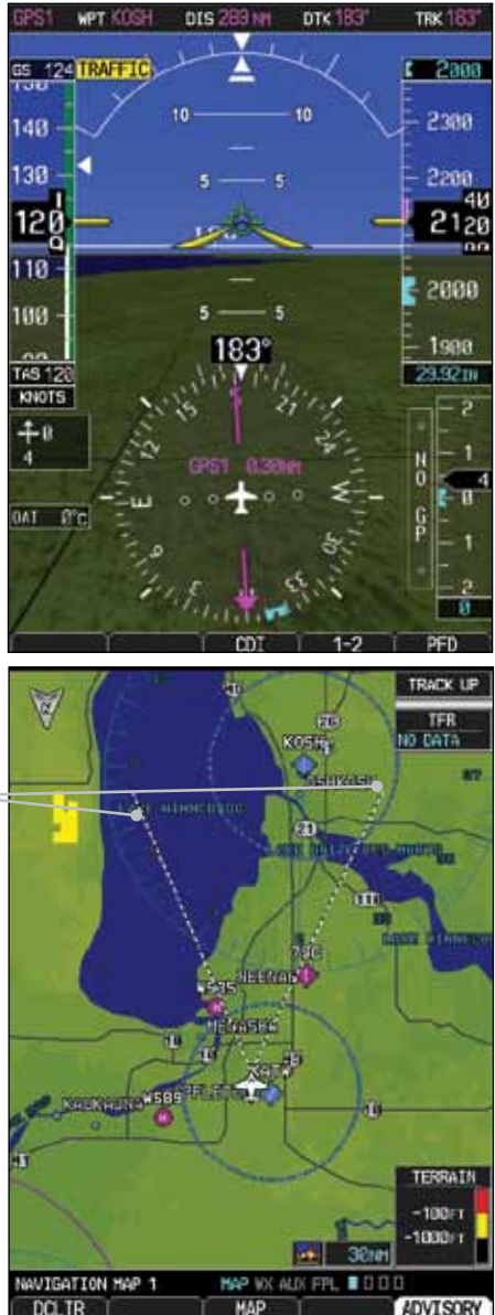
Figure 5-48 MFD and PFD Field of View Comparison
