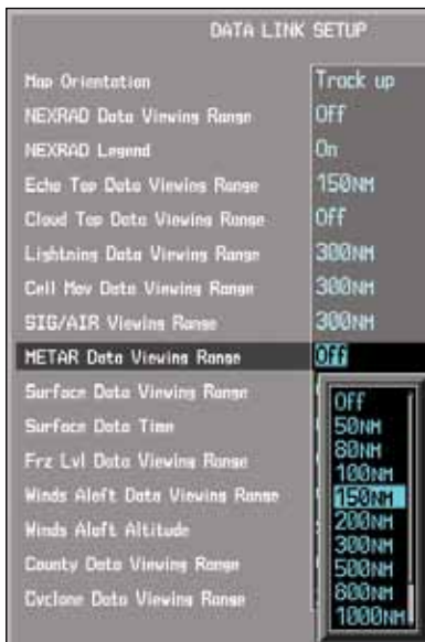
Figure 4-40 METAR Viewing Range Selection
