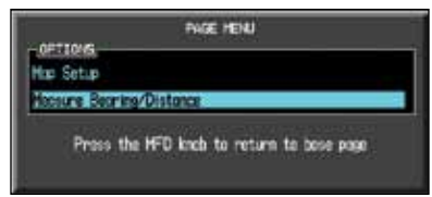
Figure 3-10 Navigation Map Measure Distance Function
