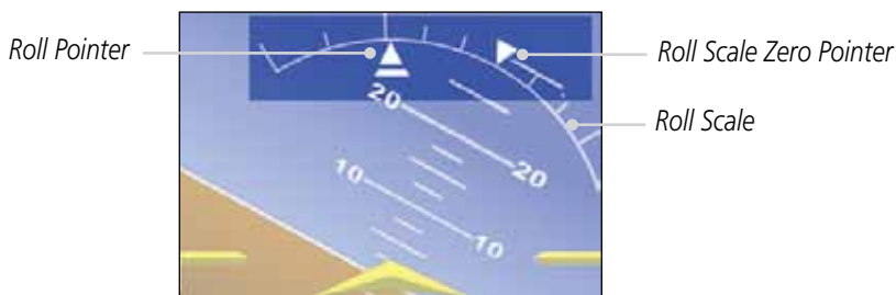
Figure 2-14 Attitude Indicator with a Ground Pointer configuration in a left turn
