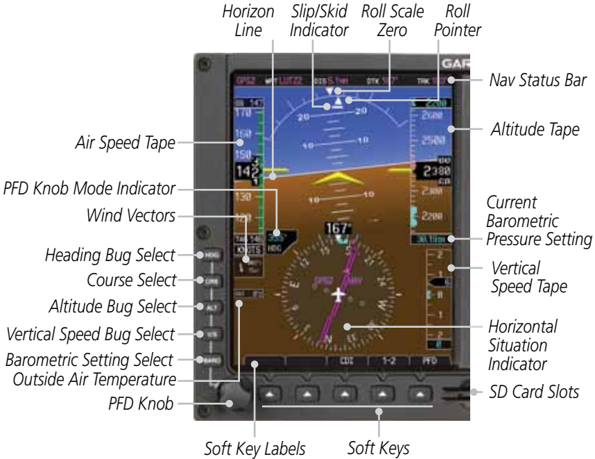
Figure 2-1 PFD Description (Ground Pointer Mode)
