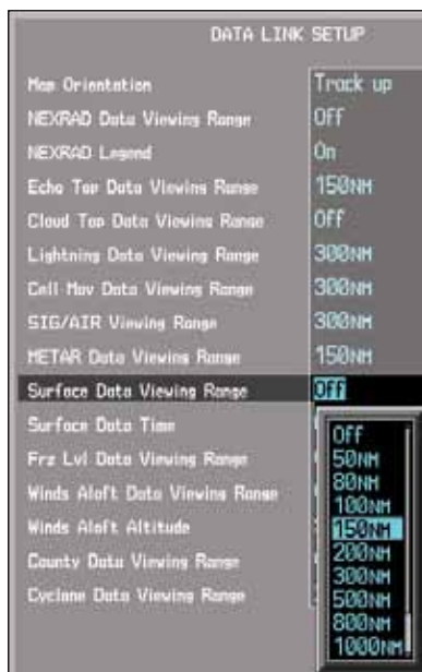
Figure 4-46 Surface data Viewing Range Selection
