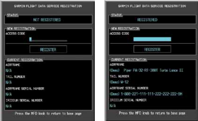
Figure 4-83 GFDS Registration Page (Default and Completed)
