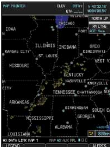
Figure 4-33 XM Weather - Lightning
