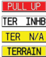
Figure 4-10 TAWS Annunciations from a GNS/GTN TAWS
