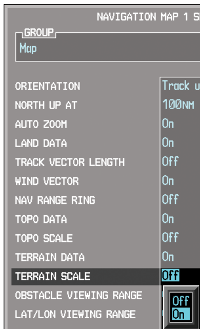
Figure 3-33 Navigation Map Terrain Scale Selection
