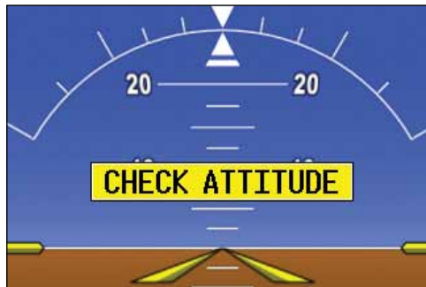
Figure 5-27 Check Attitude - Autopilot Automatically Disconnected
