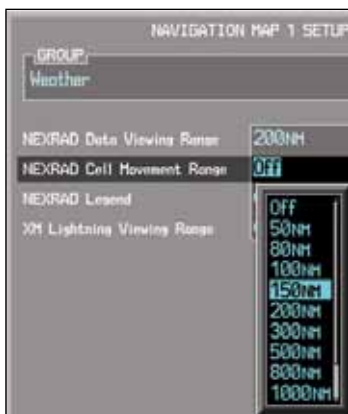
Figure 3-46 NEXRAD Cell Movement Selection
