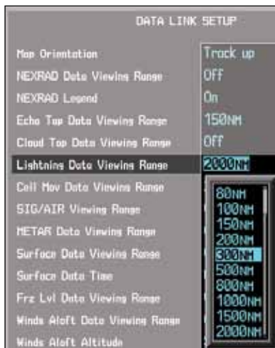
Figure 4-34 Lightning Viewing Range Selection
