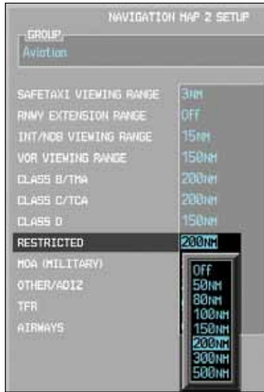
Figure 3-59 Navigation Map Restricted Airspace Viewing Range Selection
