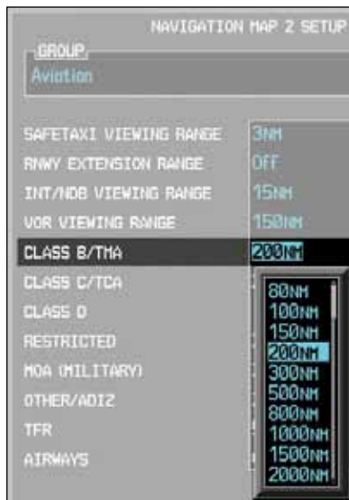
Figure 3-56 Navigation Map Class B/TMA Viewing Range Selection
