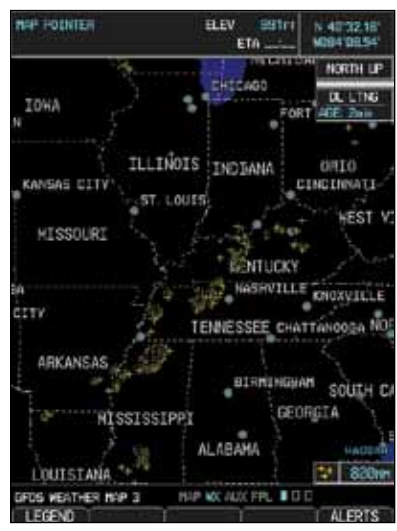
Figure 4-100 GFDS Data Link Lightning and Legend
