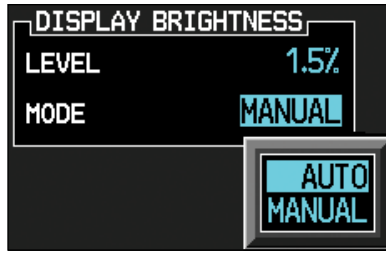
Figure 3-69 Aux Mode Display Brightness Mode Selection
