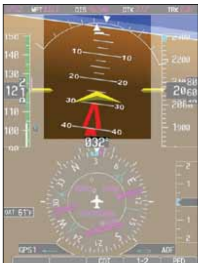
Figure 2-17 Extreme Pitch Indication Nose Down
