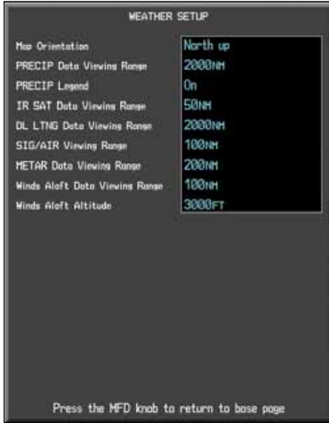
Figure 4-85 Weather Data Link Setup Menu Options
