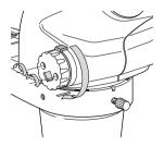
2. Set the maximum zoom level at 3.2 using the stop on the right-hand pinion knob:
