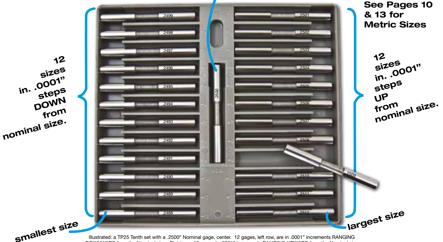
Illustrated: a TP25 Tenth set with a .2500" Nominal gage, center. 12 gages, left row, are in .0001" increments RANGING DOWNWARD from the Nominal size. Right row, 12 gages in .0001" increments RANGING UPWARD from the Nominal size
