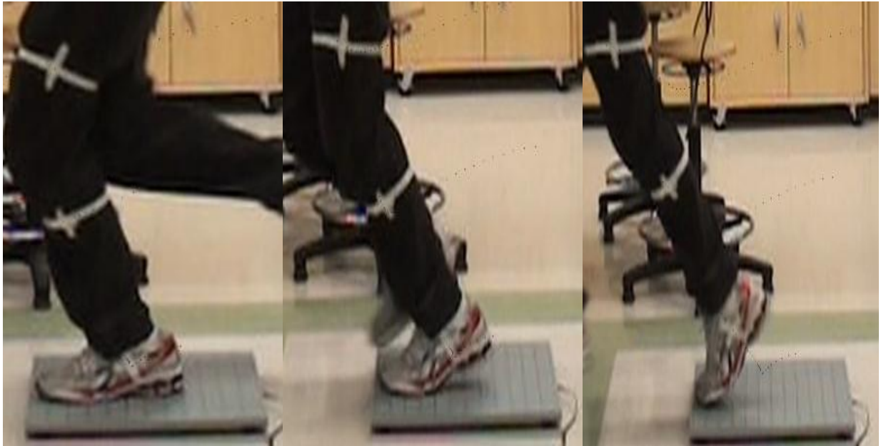
Figure 22: The test subject initially made contact with his heel on the force plate. From there the body weight is shifted forward, known as load response. The third image is the beginning of mid stance.
