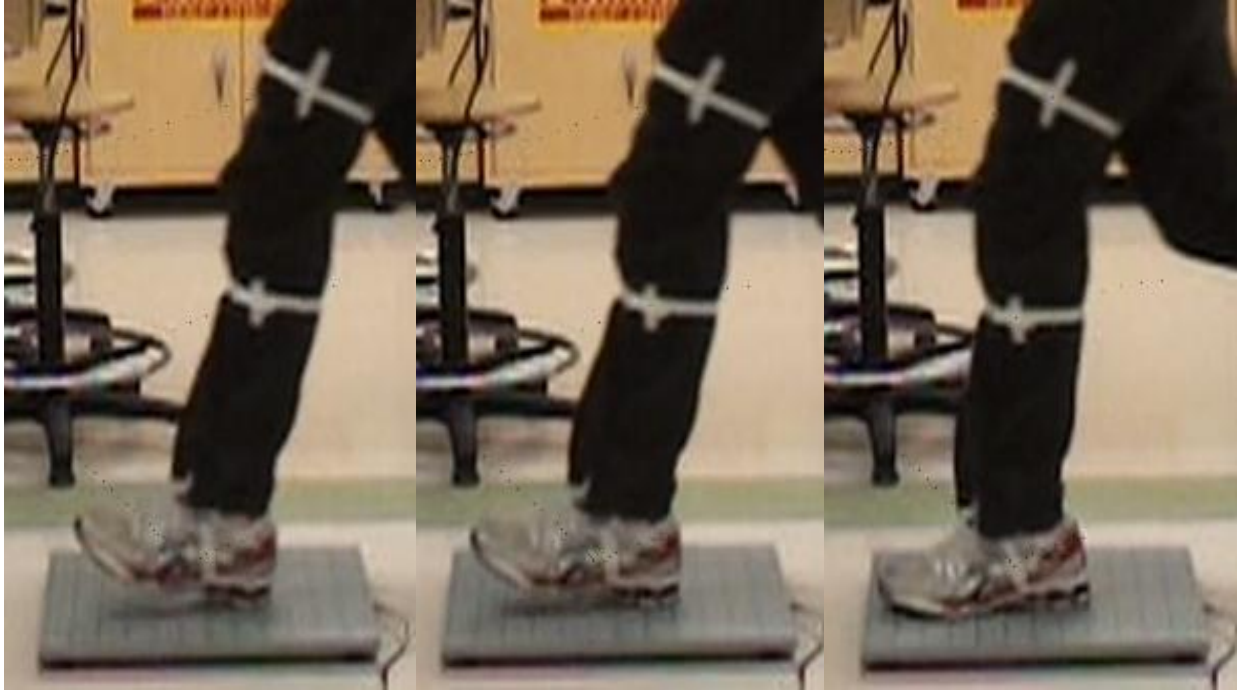
Figure 22: The test subject initially made contact with his heel on the force plate. From there the body weight is shifted forward, known as load response. The third image is the beginning of mid stance.
