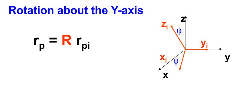
$$R = \begin{bmatrix} \cos\phi & 0 & \sin\phi \\ 0 & 1 & 0 \\ -\sin\phi & 0 & \cos\phi \end{bmatrix}$$
