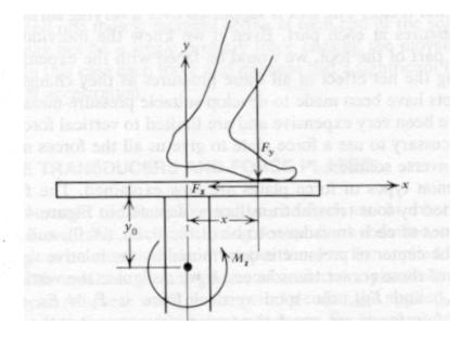
A flat plate supported by four triaxial transducers
