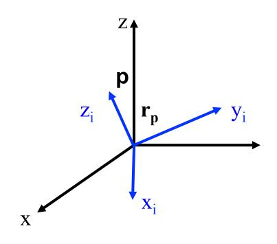
If directions of the  $x_i$ ,  $y_i$ , and  $z_i$  of the LCS axes can be expressed by unit vectors  $v_1$ ,  $v_2$ , and  $v_3$ , respectively, in the GCS, the rotation matrix from the LCS to GCS is defined as **R**
