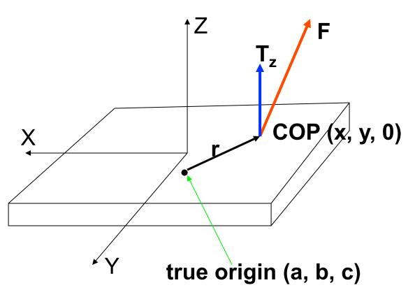
The moment measured from the plate is equal to the moment caused by **F** about the true origin plus  $T_z$ .
