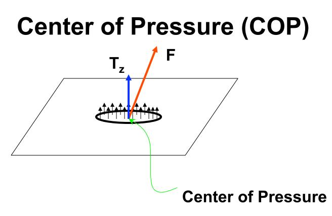
All the forces acting between the foot and the ground can be summed and yield a single reaction force vector (F) and a twisting torque vector ( $T_z$  about the vertical axis). Under normal condition there is no physical way to apply  $T_x$  and  $T_y$ .
