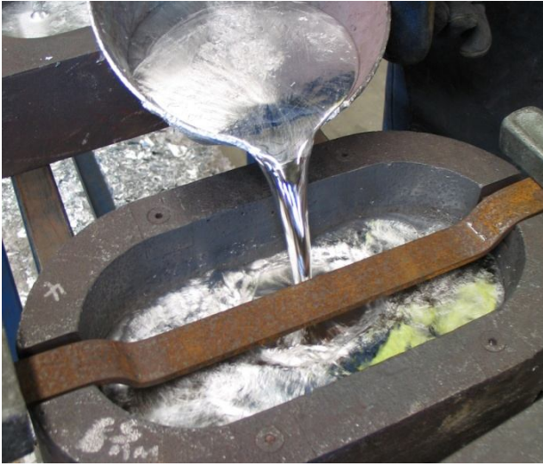
Figure 11: Casting zinc onto a corroded steel insert
