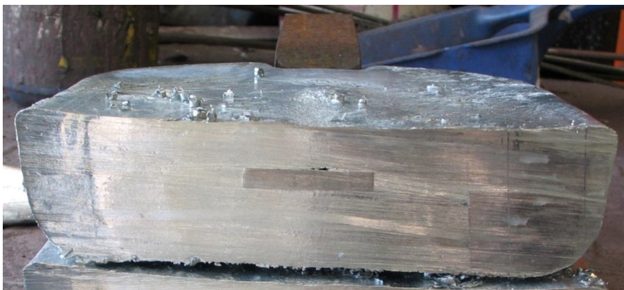
Figure 13: Destructive Test of Anode with Corroded Steel Insert
