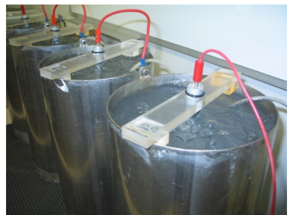
Figure 5: DNV-RP-B401 Electrochemical Testing Baths
