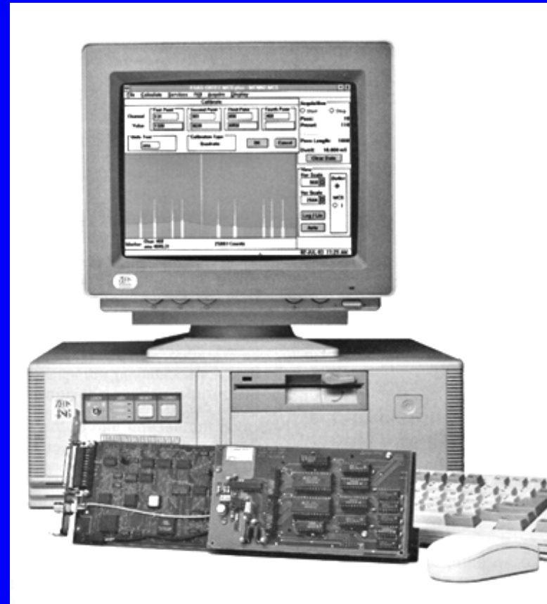
MCA's hardware on computer circuit board (old system design)
