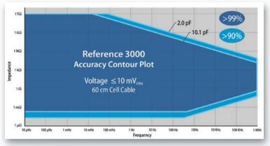
With on-board electronics for electrochemical impedance spectroscopy, the Reference 3000 can make accurate measurements over a frequency range from 10  $\mu$ Hz to 1 MHz. Modes include potentiostatic, galvanostatic, and a unique hybrid mode where potentiostatic EIS is run galvanostatically to ensure you don't accidentally damage your sample.
