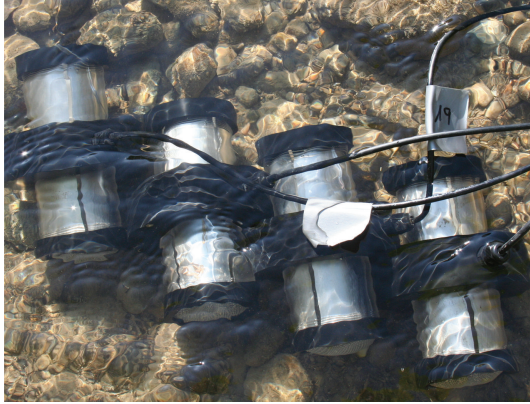
FIGURE 2: Experimental setup in situ (Photo: A. Gerhardt). View from top: four test chambers (15 × 5 cm) are placed on the sediment of the stream in flow direction, attached with ropes to steel poles in the sediment and on the banks. Each chamber contains 10 gammarids and 2 elder leaves. The test chambers can be connected to the MFB.
