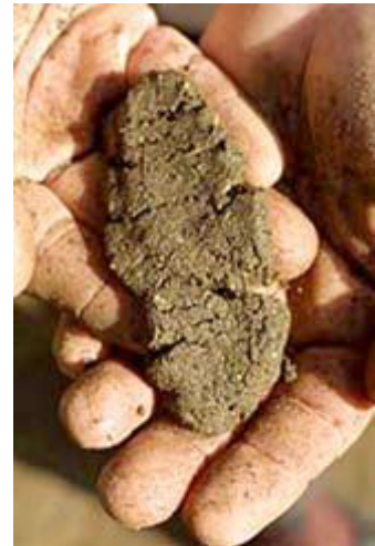
The extent of soil cracking indicates the mix of clay and sand. This example will not bend much.
