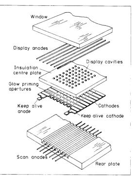
Figure 3 Exploded view of Burroughs Self-Scan panel
