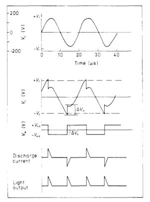
**Figure 4** The sustainer voltage  $V_s$ , tube voltage  $V_c$  and wall voltage  $V_w$  for a typical AC plasma panel together with current and light output waveforms
