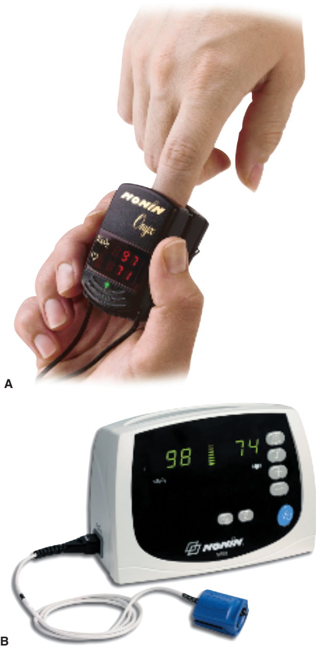
Figure 21-12 Measuring blood oxygenation with pulse oximetry reduces the need for invasive procedures, such as drawing blood for analysis of oxygen levels. A , Self-contained digital fingertip pulse oximeter, which incorporates the sensor and the display into one unit. B , Table top model with sensor attached. Memory permits tracking heart rate and oxygen saturation over time.
