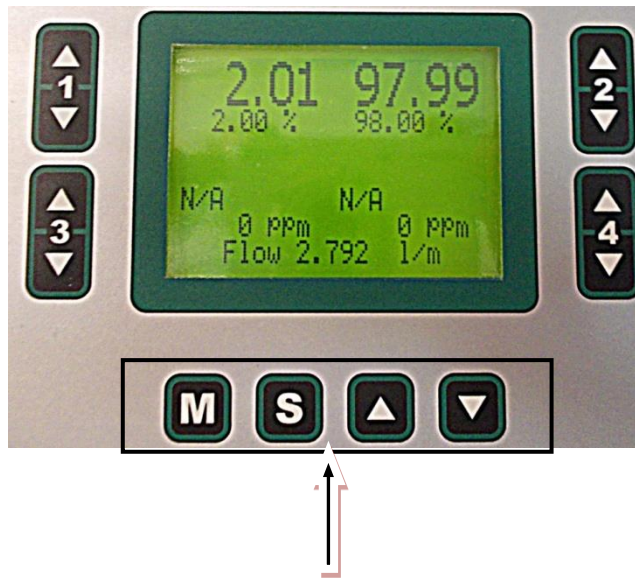
Fig. 15 Keys for operation with Menu
