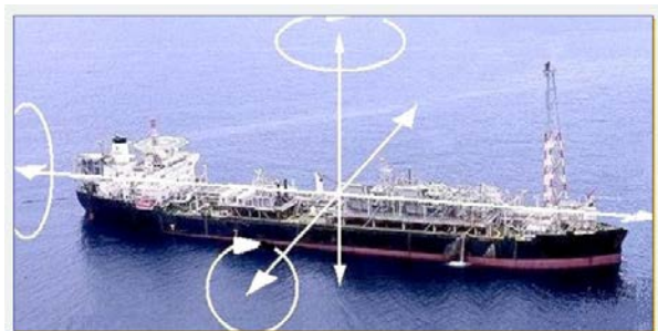
Figure 19. Degrees-of-Freedom for Dynamic Movement and Static Displacement
