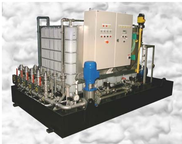
Figure 50. Typical On-Line and Off- Line Wash Skid (Courtesy of Turbotect Ltd.)
