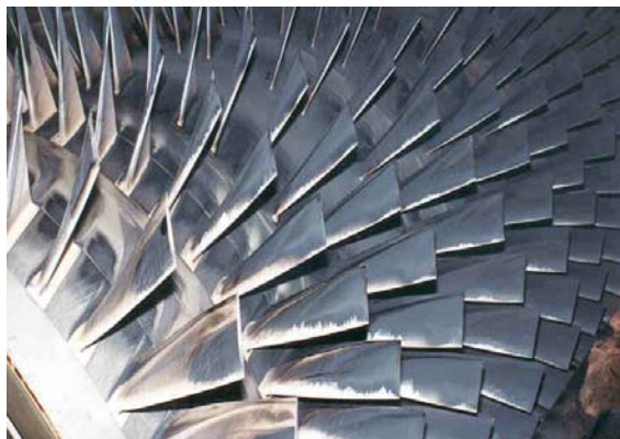
Figure 41. Axial Compressor Washed On-Line every 4-Days during 1-Month Continuous Operation.
