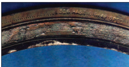
Oxidised spiral wound gasket
