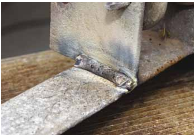
Weld on galvanised has slag...
