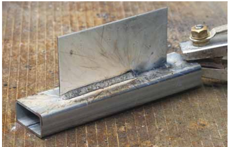
Weld on galvanised...
