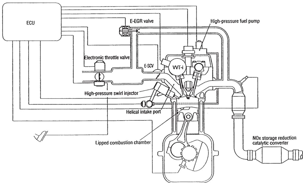
**Figure 29-19** Gasoline direct injection (GDI). Note the high-pressure swirl fuel injector at the combustion chamber. (Courtesy Toyota Canada Inc.)
