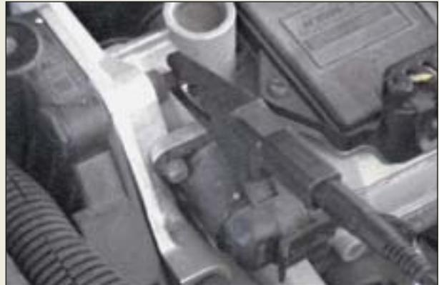
**P20-8** Attach the ground test lead to a good, clean engine ground.
