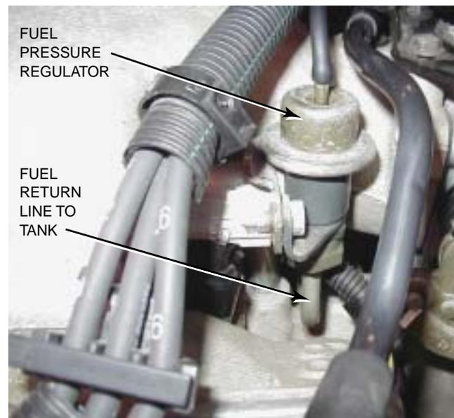
**Figure 29–25** Fuel should be heard returning to the fuel tank at the fuel return line if the fuel pump and fuel pressure regulator are functioning correctly.
