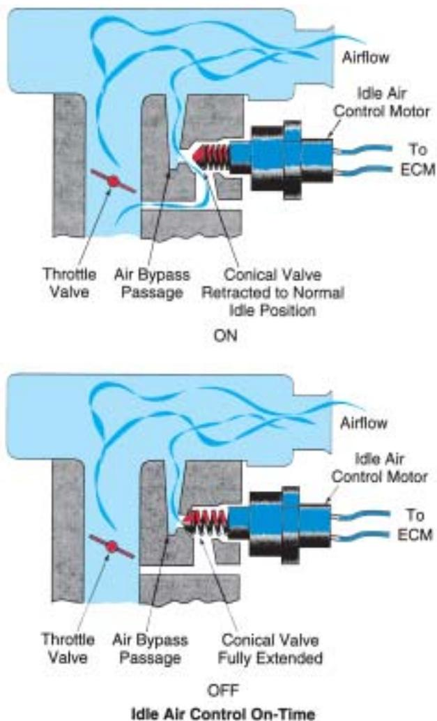
**Figure 29-35** An idle air control (IAC) controls idle speed by controlling the amount of air that passes around the throttle plate. More airflow results in a higher idle speed. (Courtesy of Fluke Corporation)
