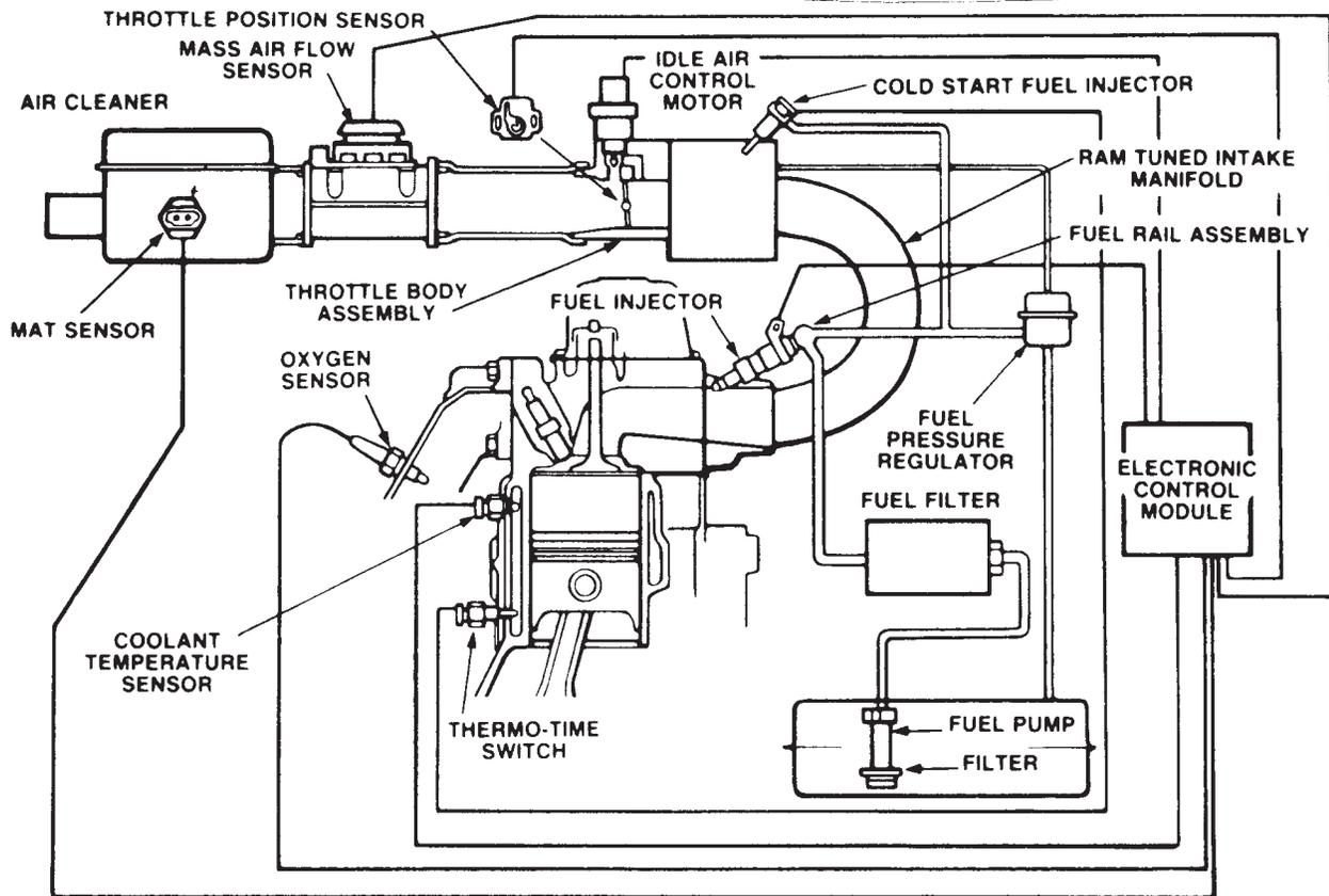
**Figure 29–42** Schematic of a General Motors 2.8 litre gasoline fuel injection system with a mass airflow sensor. Many European and Asian vehicles use a cold-start fuel injector (as does this vehicle); however, cold-start injectors are not common in domestic vehicles, which typically use a major increase in injector pulse-width (“on” time) or a primer pulse (extra injector pulse) for cold engine starting. (Courtesy General Motors)
