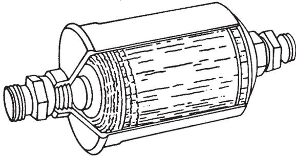
**Figure 29-3** The fuel filter is located between the fuel pump and the fuel rail. Many filters are directional and have an arrow (or different sized fittings) to prevent incorrect installation. Most systems also have a filter “sock” at the fuel tank pick-up. (Courtesy Robert Bosch)
