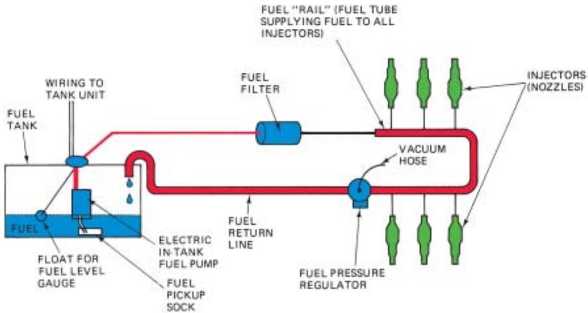
**Figure 29-1** Typical port fuel-injection system, indicating the location of various components. Notice that the fuel pressure regulator is located on the fuel *return* side of the system. The computer does not control fuel pressure, but does control the operation of the electric fuel pump (on most systems) and the pulsing on and off of the injectors.
