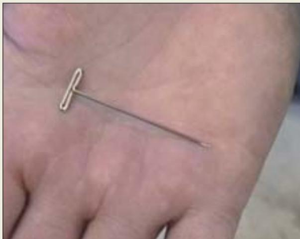
**P20-5** Use a T-pin to backprobe the injector connector. These T-pins are usually available at discount stores and specialty shops in the craft area.
