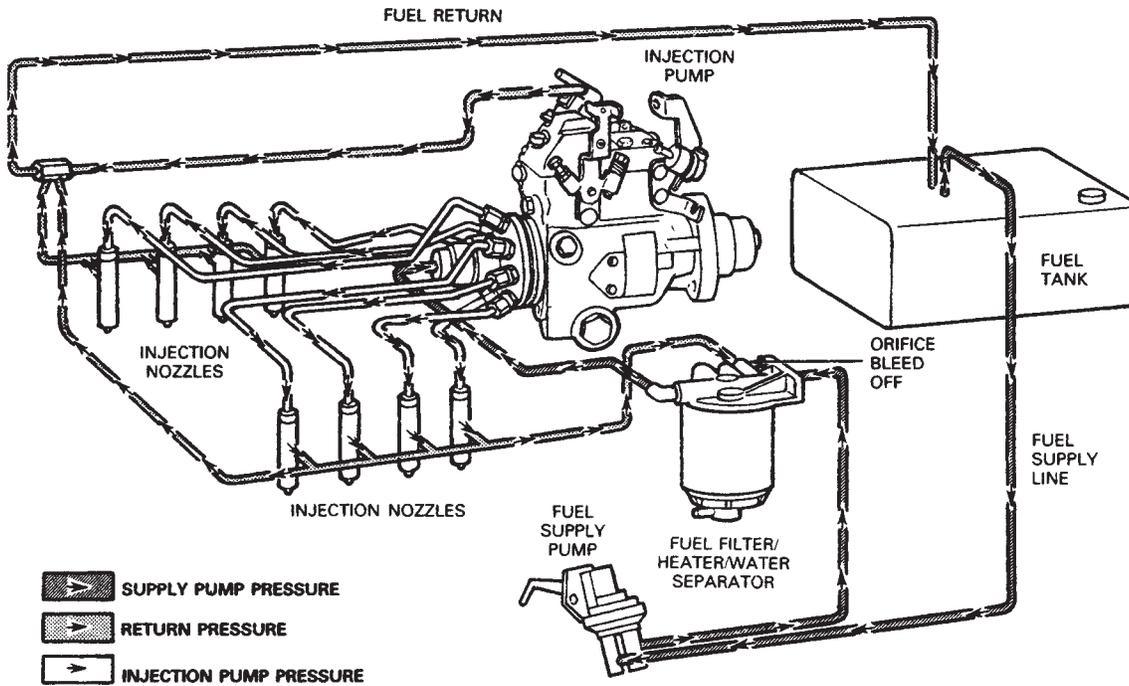
**Figure 29-44** Schematic of the fuel delivery and return on a conventional (mechanical) diesel fuel injection. (Courtesy Ford Motor Co.)
