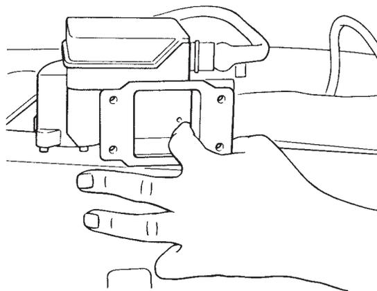
**Figure 29-20** The vane airflow meter plate should open with light pressure to the fully open position and return to rest without dragging or binding. Many European and Asian vehicles (to mid-1990s) also incorporate fuel-pump safety contacts; opening the plate with a finger (engine key “on”) will activate the fuel pump. Domestic vehicles with this type of meter use a tach signal, instead of contacts, for pump control. (Courtesy Robert Bosch)
