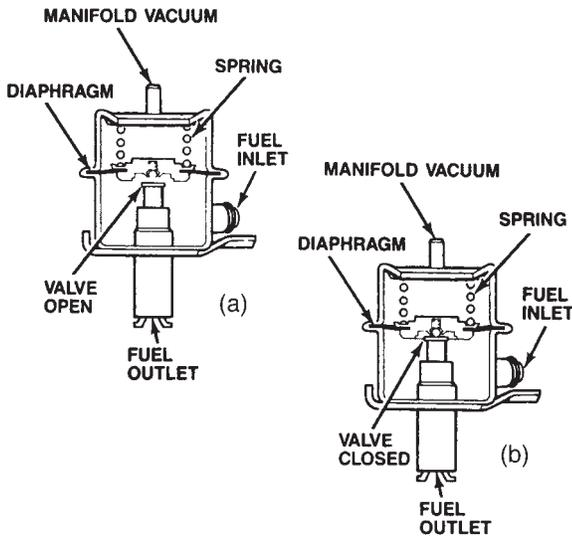
**Figure 29-7** The vacuum-modulated pressure regulator controls system fuel pressure with a spring-loaded diaphragm. (a) Strong manifold vacuum (closed throttle) works against the spring and fuel pressure decreases. (b) As manifold vacuum drops (throttle opens), full spring pressure is now exerted on the diaphragm and fuel pressure rises. (Courtesy DaimlerChrysler Corporation)
