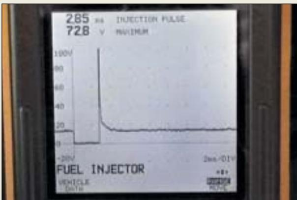
**P20-11** Note the shortened pulse width compared to the previous photo. The engine is now at normal operating temperature and the injector pulse width should be 1.5 to 3.5 milliseconds. Also look for consistent inductive voltage spikes for all injectors, indicating that the injector coil is not shorted.
