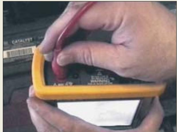
**P20-4** The scopemeter will prompt you to connect the test lead into the input A terminal.
