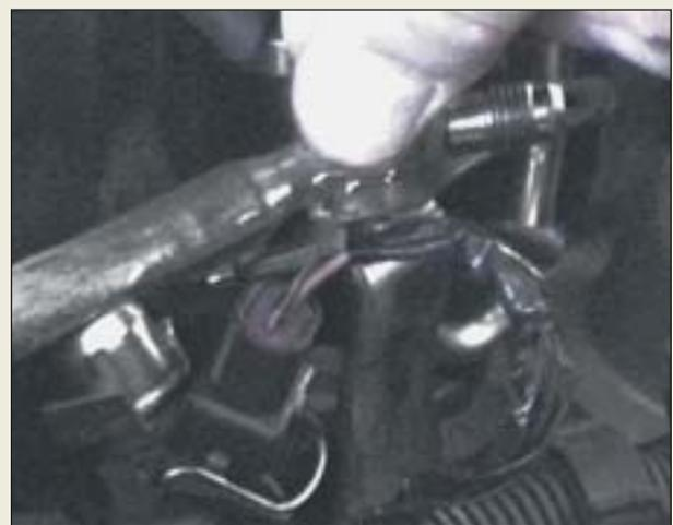
**P20-6** Carefully insert the point of the T-pin into the back of the connector and lightly push on the T-pin until it contacts the metal terminal inside the connector.
