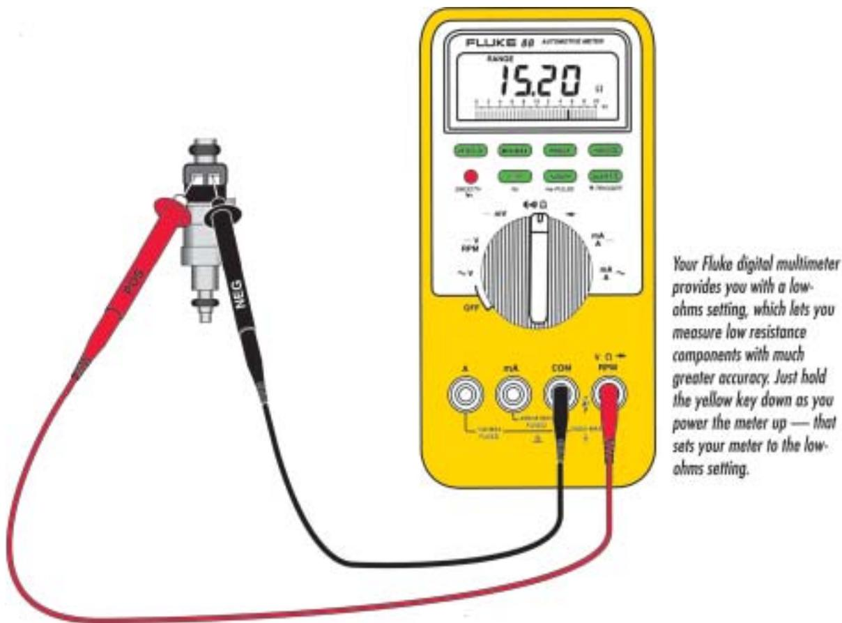
**Figure 29–27** Connections and settings necessary to measure fuel-injector resistance. (Courtesy of Fluke Corporation)
