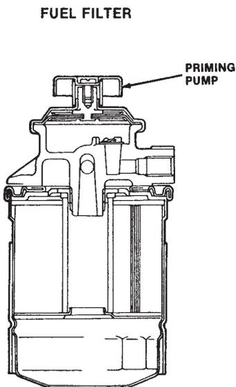
**Figure 29-45** A diesel fuel filter with built-in priming pump. (Courtesy Ford Motor Co.)
