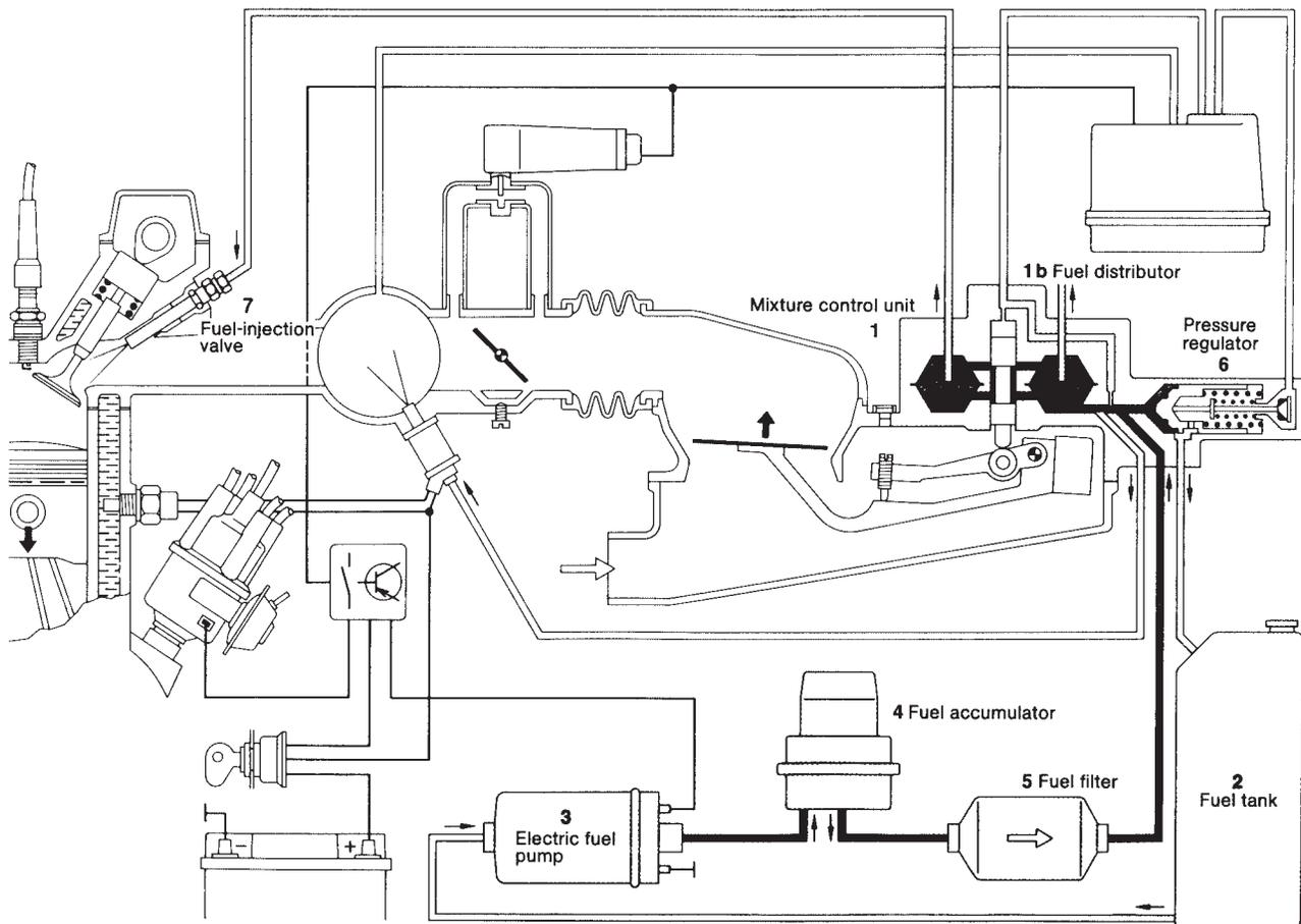
**Figure 29-14** Schematic of a Bosch CIS mechanical injection system. These units are found only on European vehicles. (Courtesy Robert Bosch)
