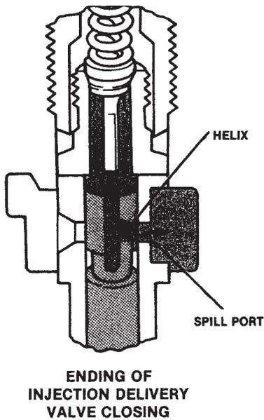
**Figure 29-52** The helix controls fuel volume by varying the opening to the spill port. (Courtesy Ford Motor Co.)
