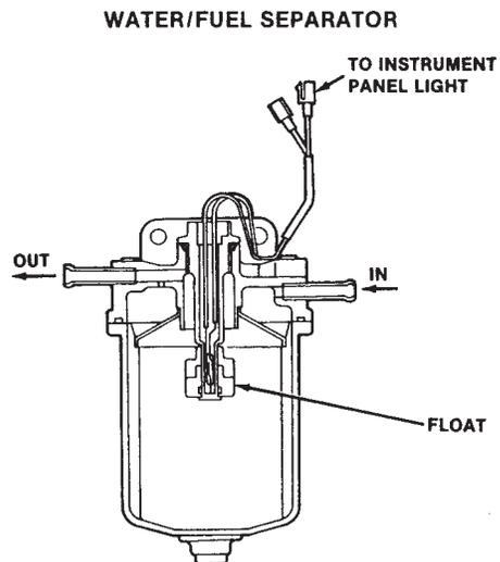
**Figure 29-46** A water/fuel separator with a water level warning light. (Courtesy Ford Motor Co.)
