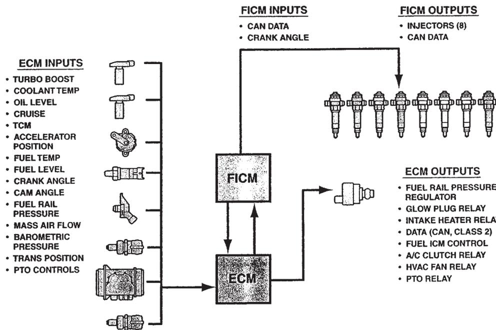
**Figure 29–59.** Diesel engine electronic management. Note the input sensors and the output actuators. (Courtesy General Motors)
