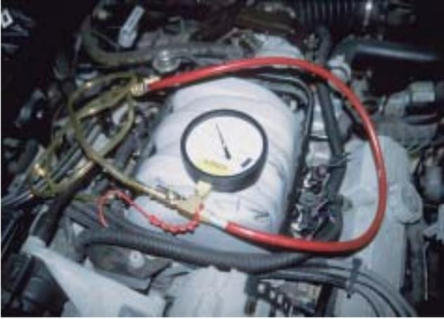
**Figure 29-22** A fuel pressure gauge connected to the fuel pressure tap (Schrader valve) on a port-injected V-6 engine.
