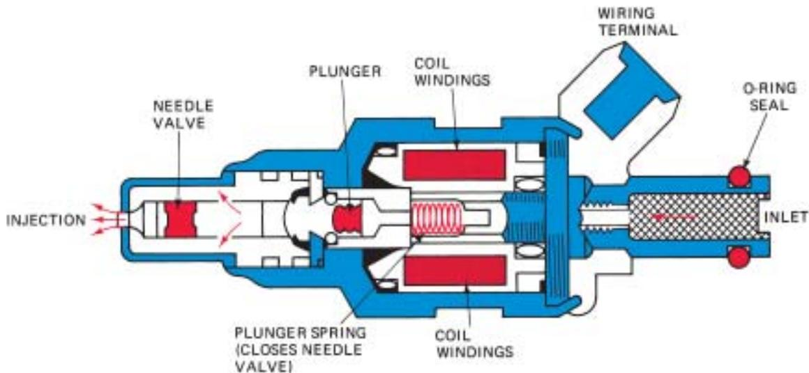
**Figure 29–5** Cross-section of a typical port fuel-injection nozzle assembly. These injectors are serviced as an assembly only; no part replacement or service is possible other than cleaning or external O-ring replacement. Contamination at the needle valve area is a common problem, especially with older type injectors. Later injectors, called deposit-resistant, changed the tip design to reduce the formation of injector deposits.
