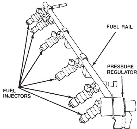
**Figure 29-4** The fuel rail is a hollow manifold that supplies fuel to the injectors. Excess fuel not used in the engine flows through a pressure regulator (usually mounted on the rail) and returns to the tank. (Courtesy DaimlerChrysler Corporation)
