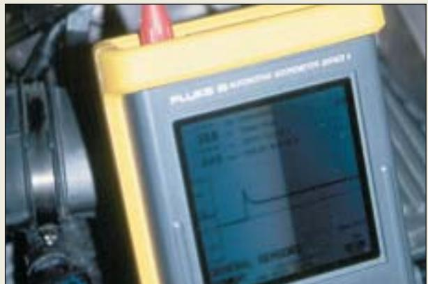
**P20-12** Turn the engine off and disconnect the scopemeter.
