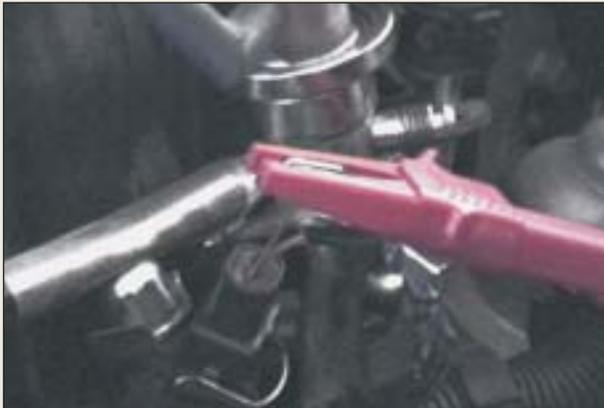
**P20-7** Attach the test probe from the scopemeter to the T-pin.
