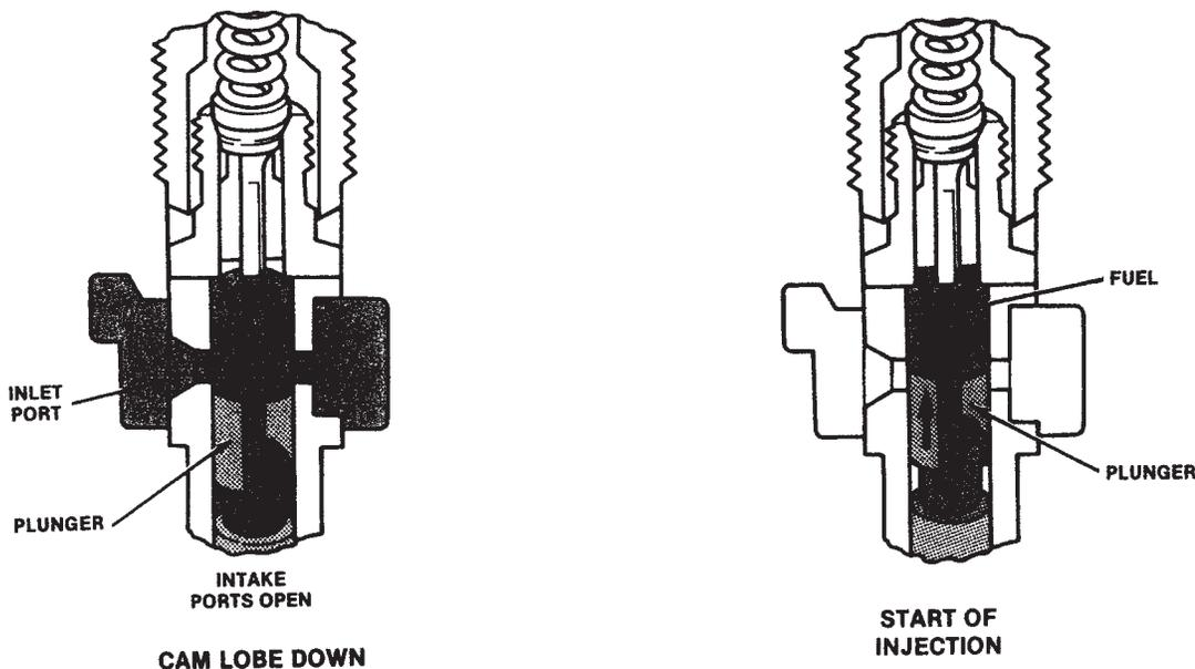
**Figure 29–48** A diesel fuel injection pump: start of injection. (Courtesy Ford Motor Co.)
