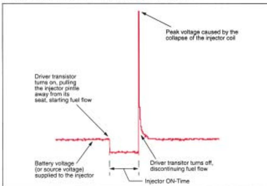
**Figure 29-30** The injector on-time is called the *pulse width*. (Courtesy of Fluke Corporation)
