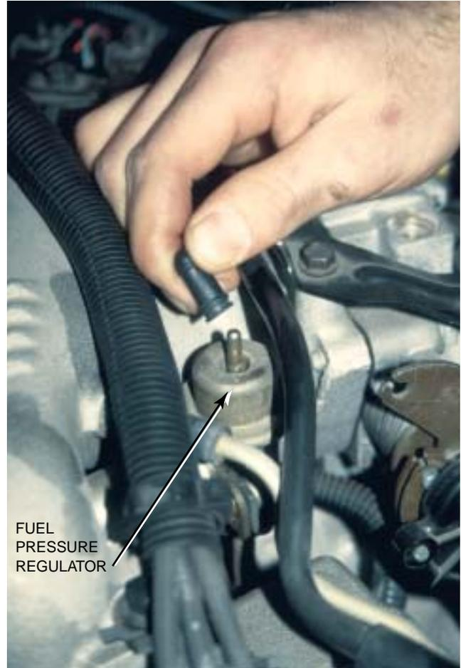
**Figure 29-23** If the vacuum hose is removed from the fuel pressure regulator when the engine is running, the fuel pressure should increase. If it does not increase, then the fuel pump is not capable of supplying adequate pressure or the fuel pressure regulator is defective. If gasoline is visible in the vacuum hose, the regulator is leaking and should be replaced.
