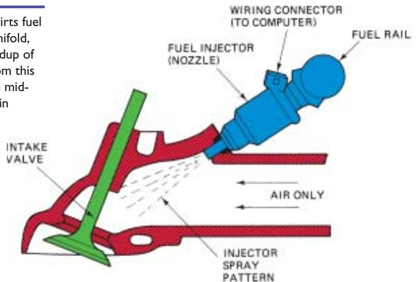
**NOTE:** Some port-injection systems used on engines with four or more valves per cylinder may use two injectors per cylinder. One injector is used all the time, and the second injector is operated by the computer when high engine speed and high-load conditions are detected by the computer. Typically, the second injector injects fuel into the high-speed intake ports of the manifold. This system permits good low-speed power and throttle response as well as superior high-speed power.
