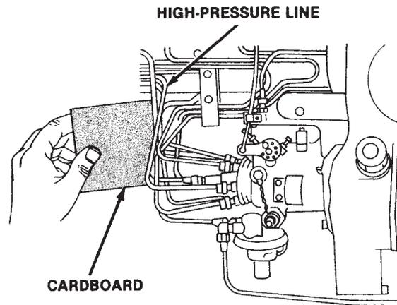
**Figure 29-50** Diesel fuel leak testing. Use cardboard to test for leaks, NEVER your hand! (Courtesy Ford Motor Co.)
