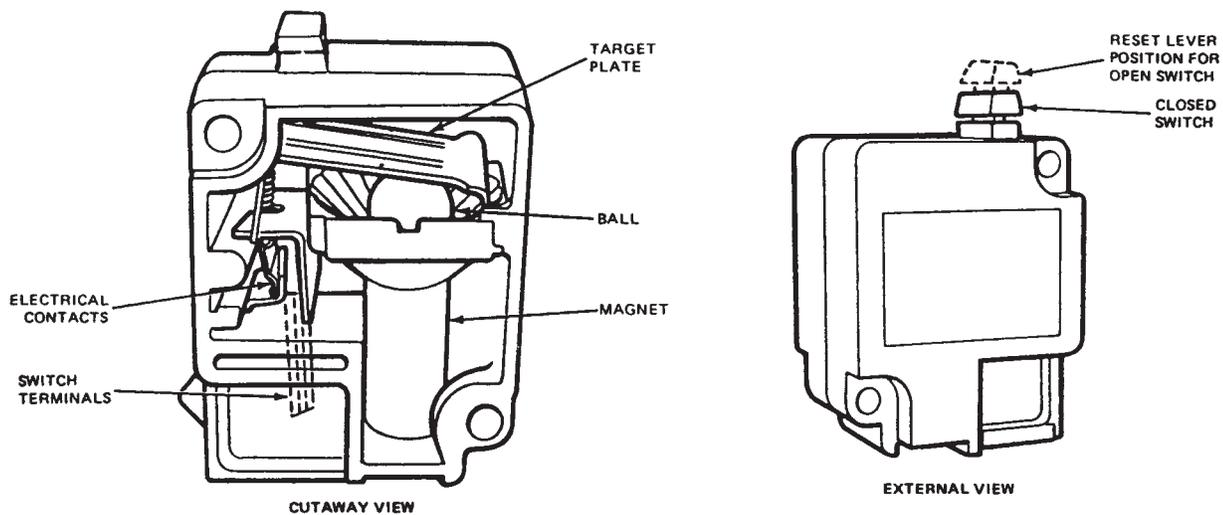
**Figure 29-10** The inertia switch is used to shut off the electric fuel pump in case of an accident. Do not reset the switch before checking for fuel leaks at the tank, lines, or engine compartment. (Courtesy Ford Motor Co.)
