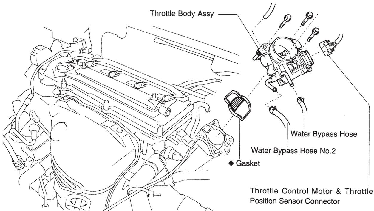
**Figure 29-38** This electronic throttle body uses engine coolant to prevent throttle plate icing. Note the location of the throttle control motor and position sensor. (Courtesy Toyota Canada Inc.)
