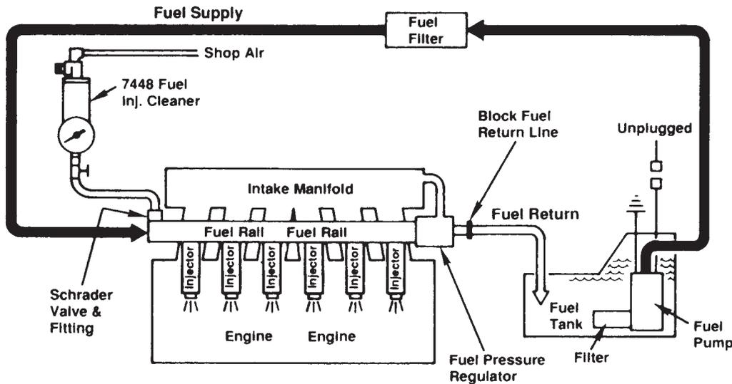
**Figure 29–33** Typical hookup for on-vehicle injector cleaning. Note the blocked fuel return line and the unplugged wiring to the fuel pump. (Courtesy OTC Division, SPX Corporation)
