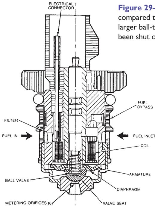
**Figure 29-13** A low-pressure TBI/CFI fuel injector feeds all cylinders compared to a port fuel injector, which feeds only one cylinder. The larger ball-type injector tip is prone to leak or drip when the engine has been shut off. (Courtesy Ford Motor Co.)
