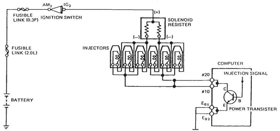
Sequential injection has a number of advantages over simultaneous injection: 1) Emissions are reduced during low RPM and idle conditions. 2) It works with waste spark ignitions that fire the spark plug every revolution. 3) OBD II systems have the ability to cancel fuel delivery to any cylinder that is misfiring. This protects the catalytic converter.
