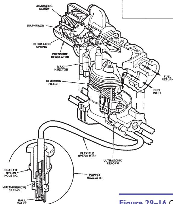
**Figure 29–16** Central port injection (CPI) operation. (Courtesy General Motors)
