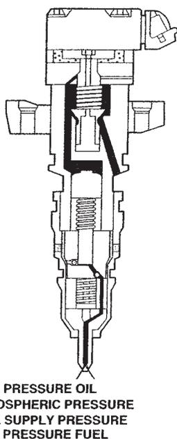
**Figure 29–60** A high-pressure solenoid controlled fuel injector. (Courtesy Ford Motor Co.)
