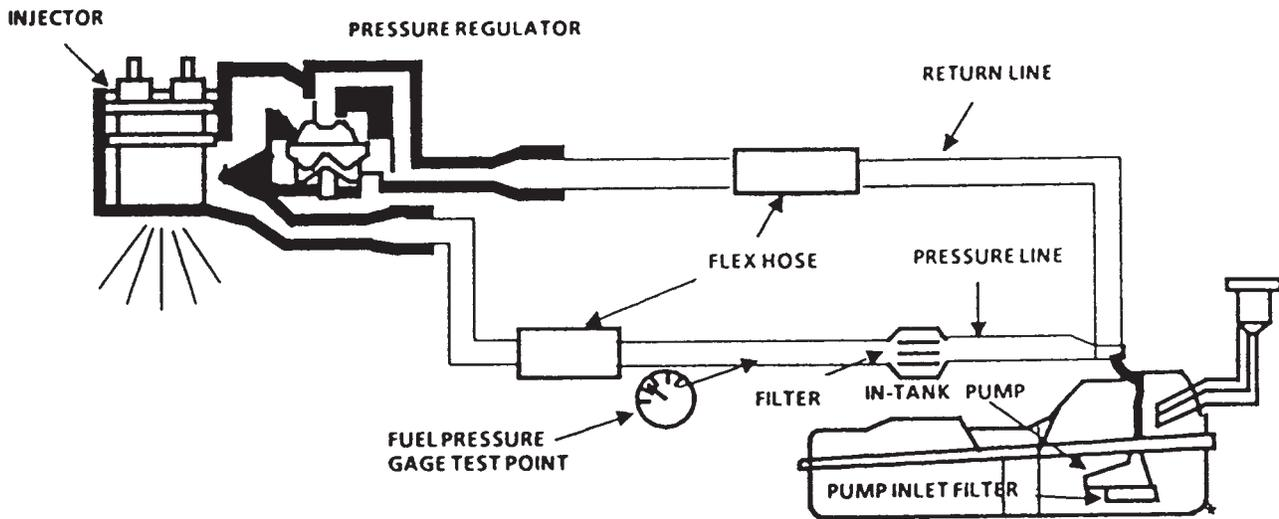
**Figure 29-12** Fuel delivery and return lines on this TBI system are similar to port fuel injection. (Courtesy General Motors)
