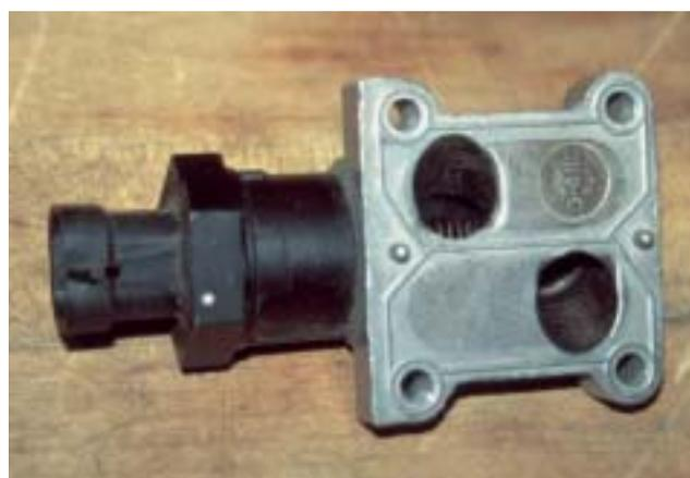
**Figure 29-37** Some idle air control units are purchased with the housing as shown. Carbon buildup in these passages can cause a rough or unstable idling or stalling.
