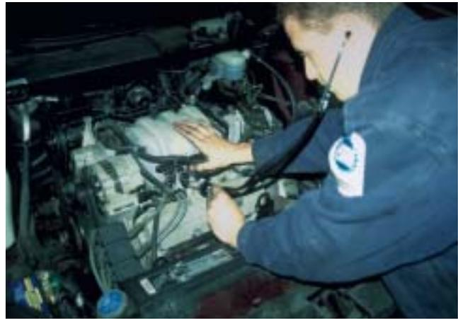
**Figure 29–24** All fuel injectors should make the same sound with the engine running at idle speed. A lack of sound indicates a possible electrically open injector or a break in the wiring. A defective computer could also be the cause of a lack of clicking (pulsing) of the injectors.
