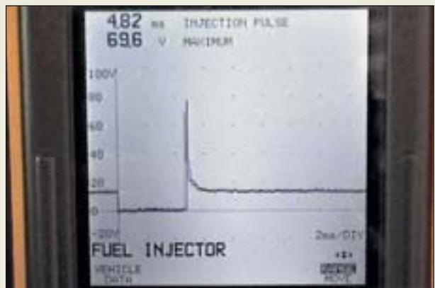
**P20-10** Observe the waveform. If the waveform does not look similar to this, insert the T-pin into the other terminal of the connector. To achieve this pattern, the scopemeter should be connected to the terminal that is being pulsed on and off by the computer. The pulse width is longer than normal in this photo because the engine is cold and the computer is pulsing the injector on for a longer time to provide the engine with additional fuel.
