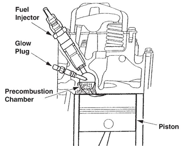
**Figure 29-56** Indirect fuel injection injects fuel into a precombustion chamber. A glow plug is used to ignite the fuel during cold engine operation. (Courtesy Ford Motor Co.)
