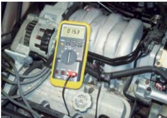
**Figure 29–28** To measure fuel-injector resistance, a technician constructed a short wiring harness with a double banana plug that fits into the V and COM terminals of the meter and an injector connector at the other end. This setup makes checking resistance of fuel injectors quick and easy.
