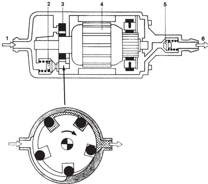
**Figure 29-2** Schematic of a roller-cell fuel pump. Note #5 non-return valve, which prevents fuel pressure from bleeding back through the pump, and #2 pressure limiter (relief) valve, which acts as a safety valve if the fuel filter or line is restricted. (Courtesy Robert Bosch)
