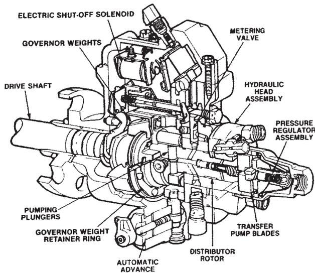
**Figure 29-54** Ghost view of a rotary diesel fuel injection pump. (Courtesy General Motors)
