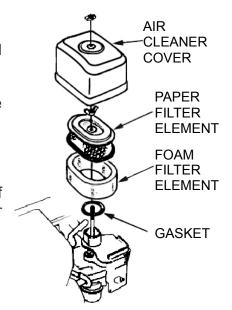
Paper air filter element: Tap the filter element several times on a hard surface to remove dirt, or blow compressed air [not exceeding 30 psi (207 kPa)] through the filter element from the inside. Never try to brush off dirt; brushing will force dirt into the fibers.
