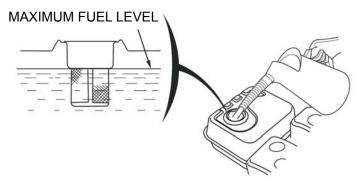
Refuel in a well-ventilated area before starting the engine. If the engine has been running, allow it to cool. Refuel carefully to avoid spilling fuel. Do not fill above the fuel strainer shoulder. After refueling, tighten the fuel tank cap securely.
