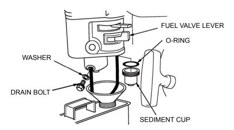
3. After all the fuel has drain into the container, reinstall the drain bolt and sediment cup. Tighten them securely.
