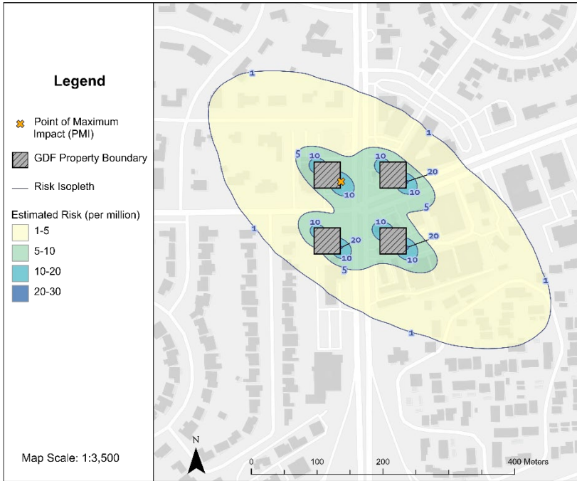
Figure A6. Zone of Impact of Gas Station Emissions: Four Three-Million-Gallon Gas Stations with 100m Separation (Urban) 1,2
