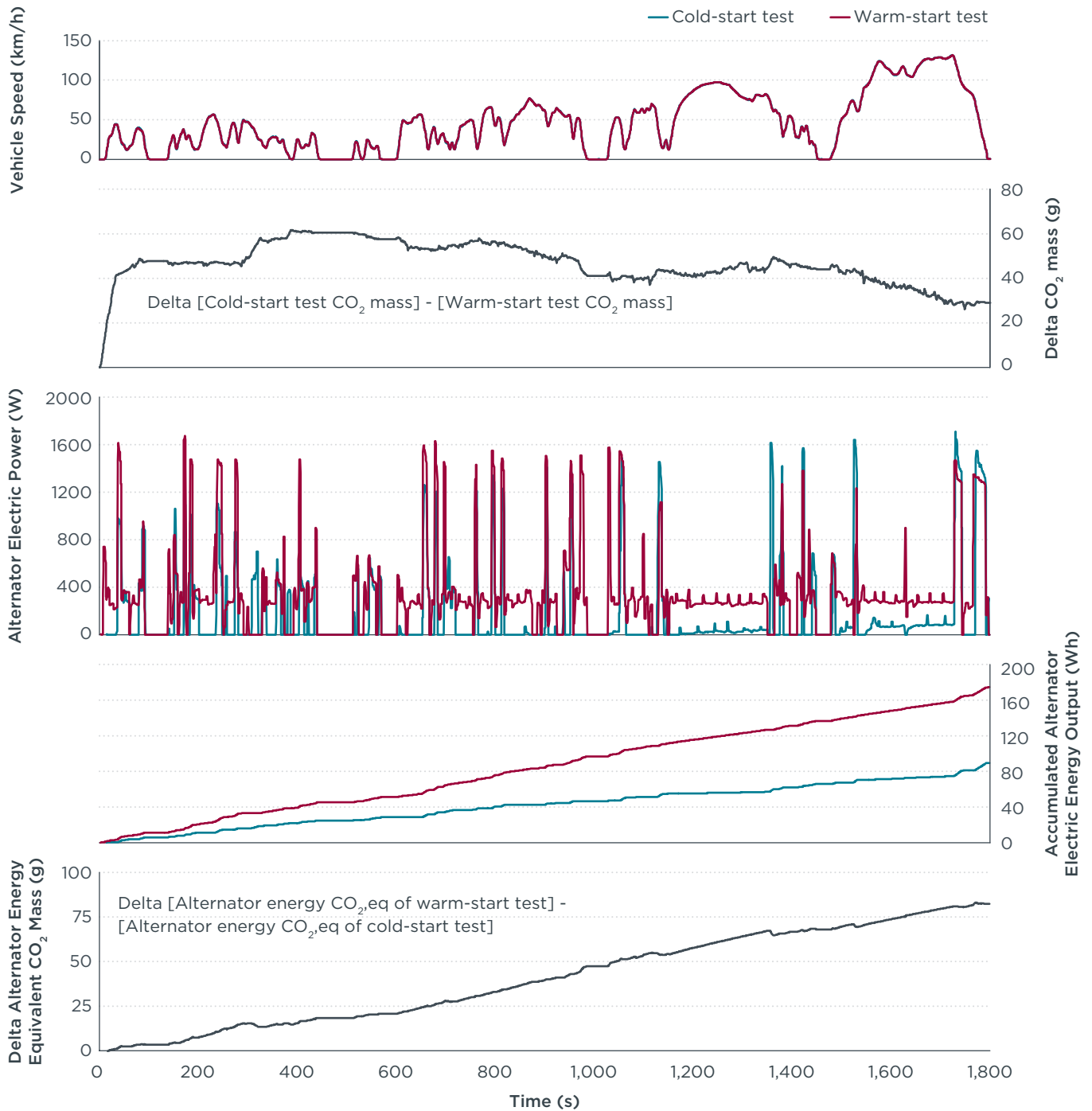
Figure 12. Golf TSI alternator power generation in cold- and warm-start WLTC at 23 °C. Alternator energy equivalent CO 2 mass is approximately 82 g higher for the warm-start than for the cold-start test.
