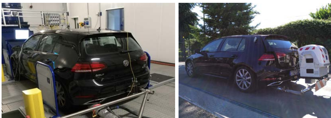
Figure 2. Golf TSI test vehicle, on chassis dynamometer and on the road with portable emissions measurement system (PEMS) installed.
