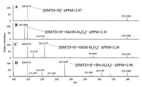
**Figure 3.** Infusion of HMTD standard solutions ( $5 \mu g/mL$ , 50:50 v/v) in (A) acetonitrile/water, (B) methanol/water, (C) ethanol/water, and (D) isopropanol/water.
