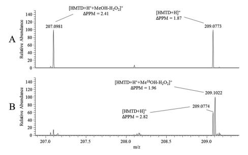
**Figure 4.** Infusion of HMTD standard solutions (5  $\mu$ g/mL, 50:50 v/v) in (A) methanol/ water and (B) [<sup>18</sup>O]-methanol/water. Circled areas are expanded insets within each spectrum.
