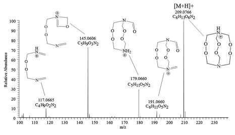
**Figure 1.** HMTD and tentatively identified fragment ions produced in the source using APCI+, with acetonitrile/water with 0.1% acetic acid mobile phase.
