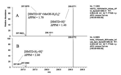
**Figure 2.** Infusion of HMTD standard solutions (5  $\mu$ g/mL) in (A) 100% methanol and (B) 10% methanol/90% water. Note that, with the 10% methanol solution, the peak associated with [HMTD-H<sub>2</sub>+H]<sup>+</sup> is ~50% of the [HMTD+H<sup>+</sup>+MeOH-H<sub>2</sub>O<sub>2</sub>]<sup>+</sup> peak, but only 5% relative abundance in both spectra.
