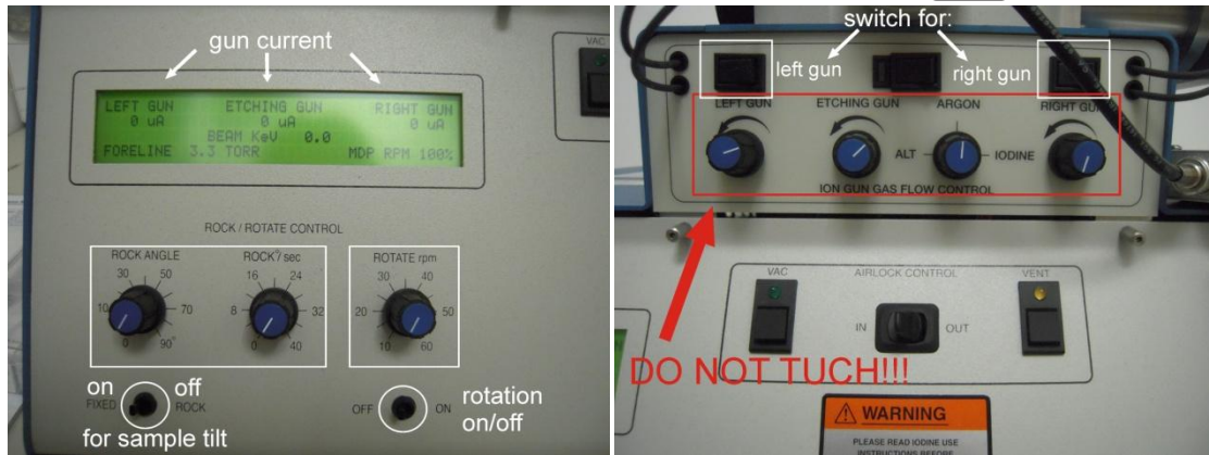
Figure 4: Left: a control panel for the rotation and tilt of the sample and current and voltage monitor on the ion guns. Right: switches for ion guns, switch "Airlock Control" and "Vent".
