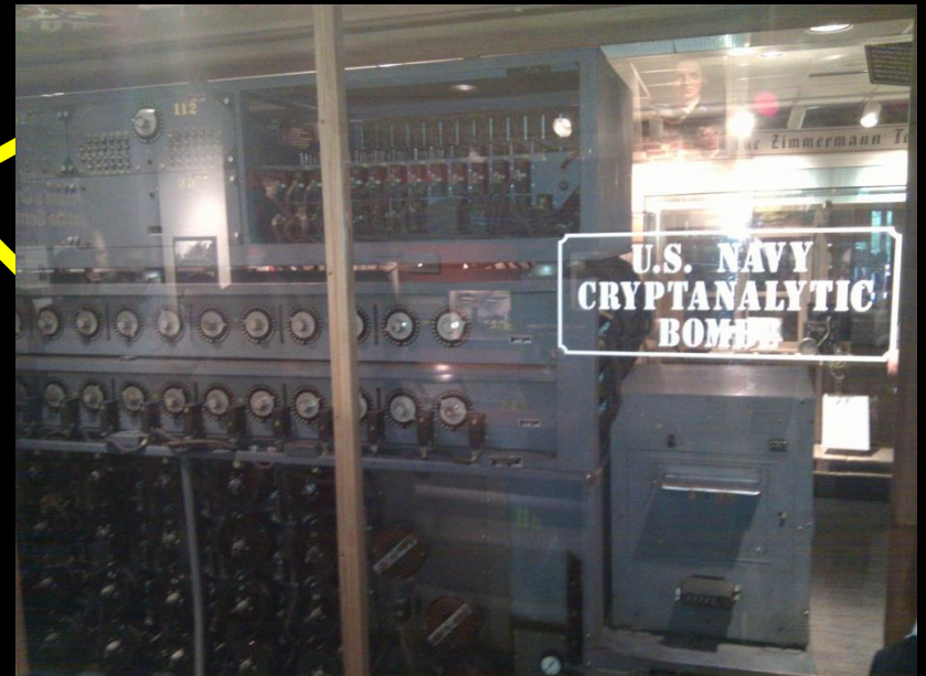
The Bombe used to break the German Enigma machine during World War II
