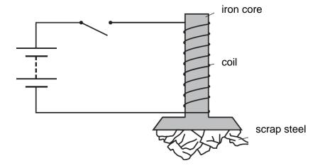
When the switch is closed, the scrap steel is attracted to the electromagnet.
