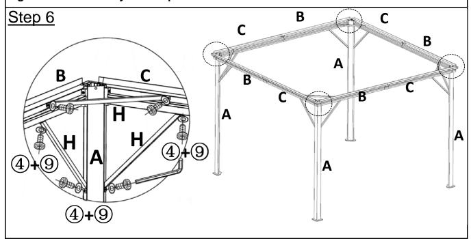
Attach Connection Piece(H) between Left Short Beam(B) and Right Short Beam(C) using Bolts(4) and Washers(9) with Allen Key(7).
