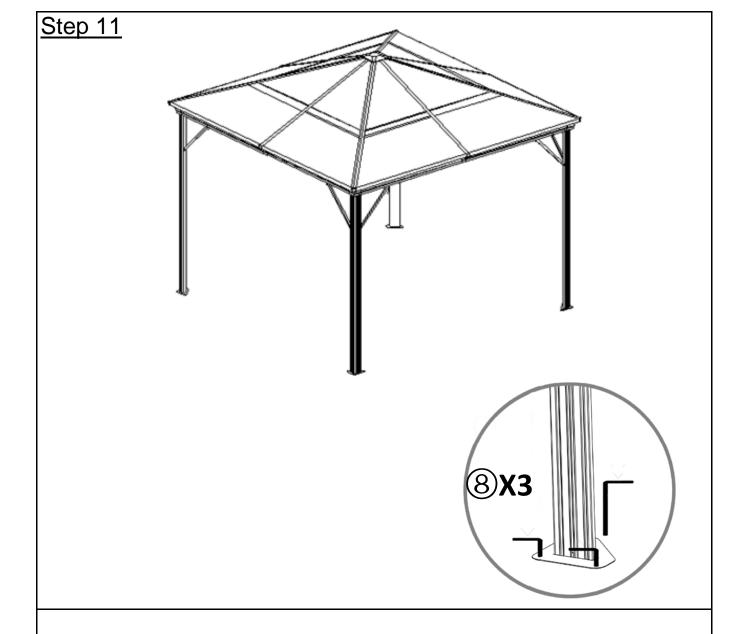
Affix the Gazebo to the ground by inserting the Stakes( $\otimes$ ) through the Bases(T). Your Gazebo is ready for use.
