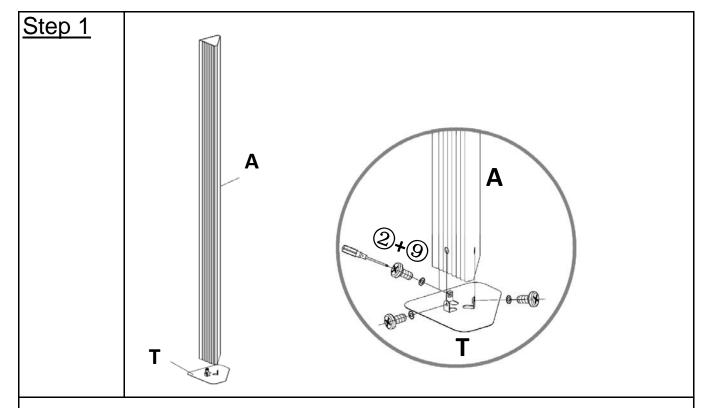
Attach Columns(A) onto Bases(T) using Bolts(2) and Washers(9) with Screwdriver(6). **Tighten the Bolts fully in a sequential manner.**
