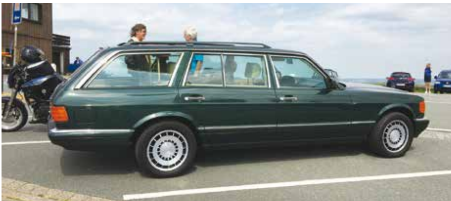
The roof rails on the Zender conversion come from a W123...
