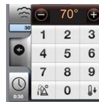
keypad for adjusting the core probe temperature
