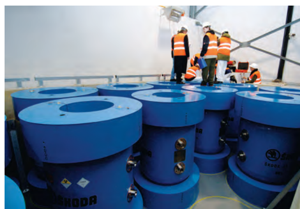
FIG. 1. Transport packages for radiation sources under preparation.
