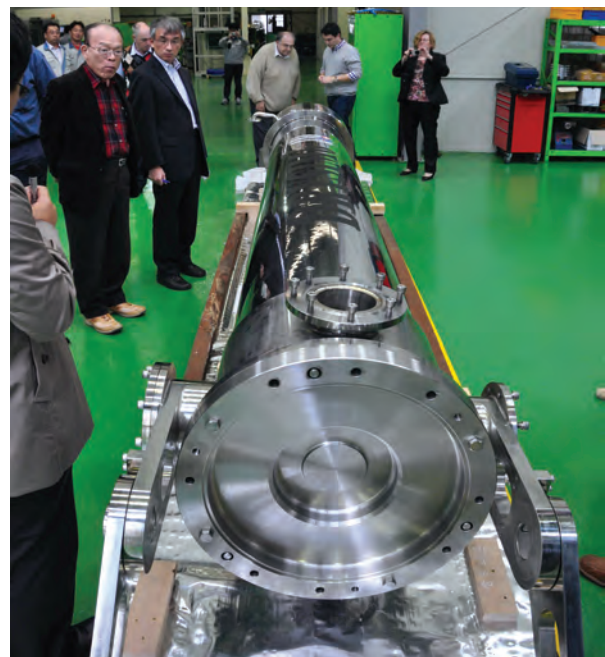
FIG. 3. Participants in the SPAR CRP inspecting the DrySim6 dry storage simulation test equipment at the Korea Atomic Energy Research Institute. (Photograph courtesy of VUJE.)
