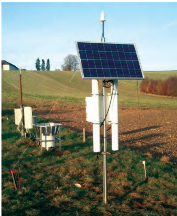
FIG. 2. Cosmic ray soil moisture system in Petzenkirchen, Austria.
