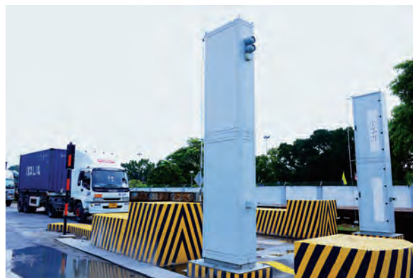
FIG. 1. A radiation portal monitor at the border between Thailand and Malaysia. This device detects radiation in real time, without interrupting normal import–export operations.
