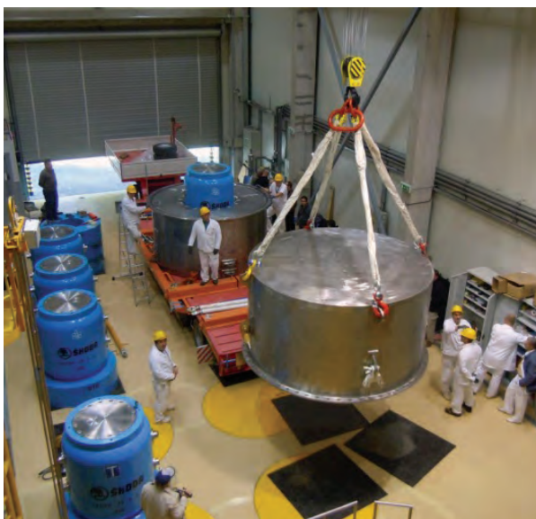
FIG. 2. Dual purpose casks (blue) procured by the Agency being loaded into TUK-145/C transport packages for the repatriation of spent HEU fuel at the KFKI Atomic Energy Research Institute research reactor site in Budapest.
