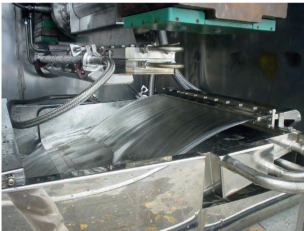
FIG. 2. Electron beam treatment of industrial wastewater to make it safer for disposal. (Photograph courtesy of EBTech.)
