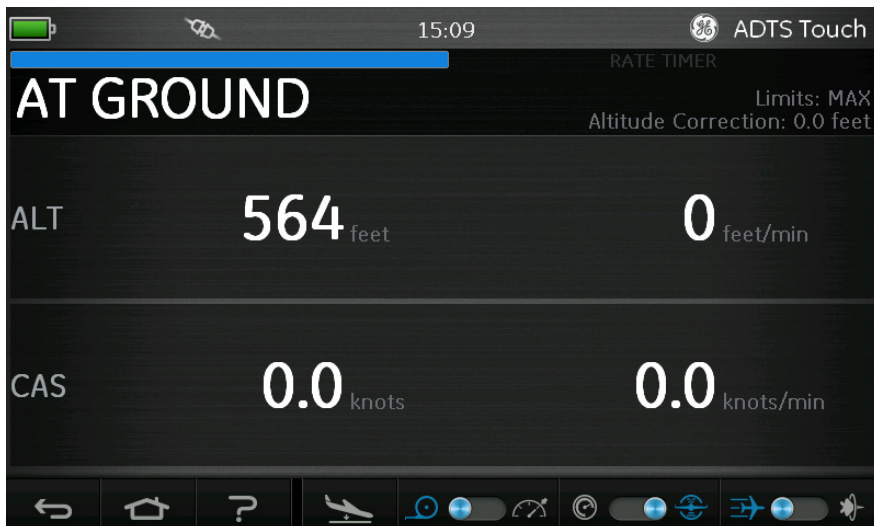
Figure 3-18 Go to ground complete
