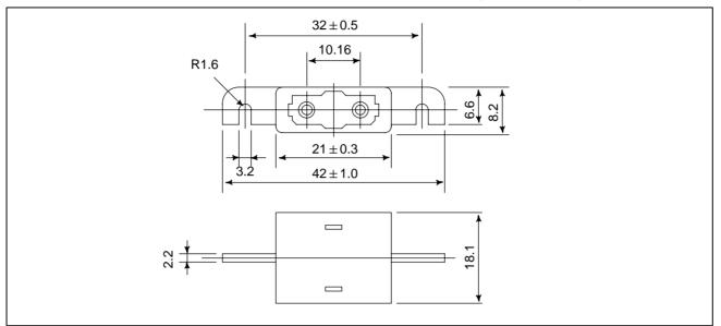
(a) External view of the low-loss optical relay adapter
