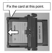
Fix the memory card to the fixing bracket.
