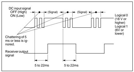
Fig. 9.7.1 (b) Signal width and delay of input signal
