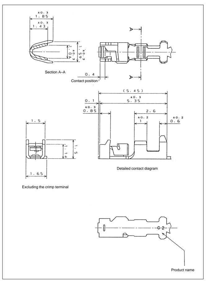
Fig. C7 (b) Contact (Japan Aviation Electronics)(for MDI)
