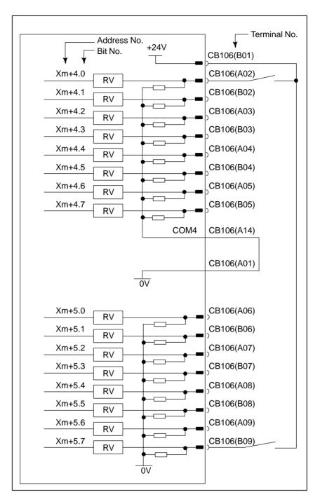
For address Xm+4, either a source or sink type (with a 0- or 24–V common voltage) can be selected. COM4 must be connected to either 24 or 0 V; never leave it open. From the viewpoint of safety standards, it is recommended that a sink type signal be used. The above diagram shows an example in which the signal is of sink type (with a 24–V common voltage).
