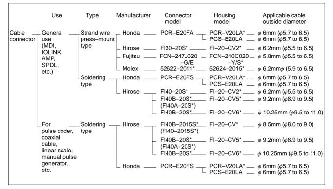
Fig. B.3 Cable connectors
