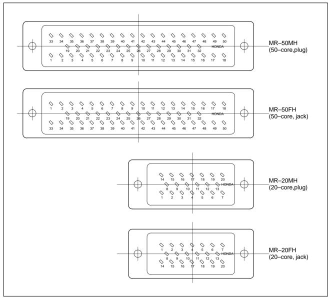
Fig. C4 (e) HONDA connector (terminal layout)
