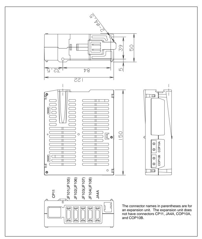
Fig.U20 External dimensions of separate detector interface unit
