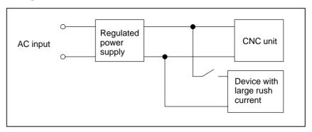
For a circuit configuration in example 2, connect another regulated power supply to be specifically used for the device with remarkable load fluctuations so that the CNC and other units are not affected.
