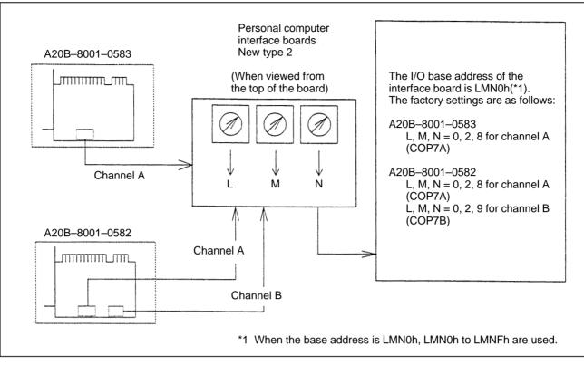
Fig. 11.6 I/O base address setting (for personal computer interface board of new type 2 (A20-B-8100-0582, -0583))
