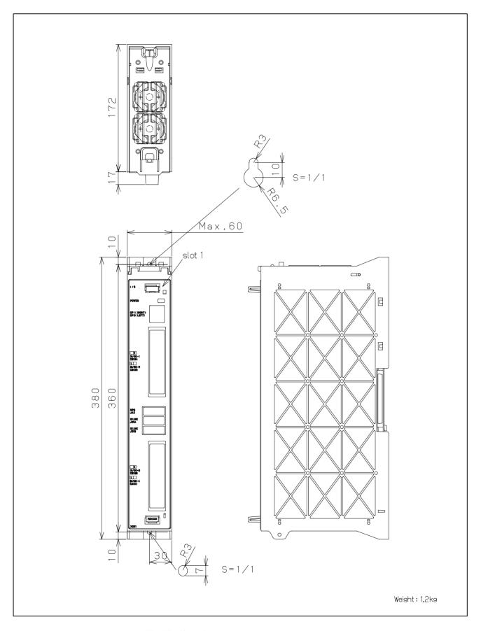
Fig.U5 I/O unit for 0*i* Specification No. : A02B–0309–C001
