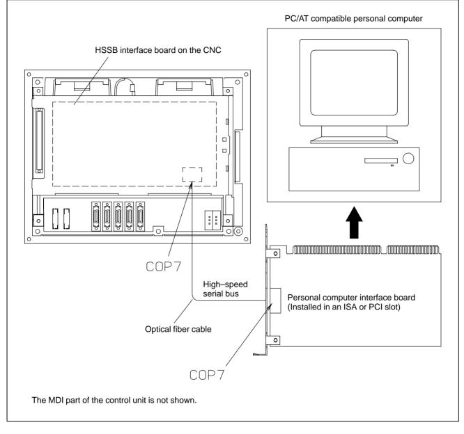
The PC interface boards include an ISA bus interface board and a PCI bus interface board.
