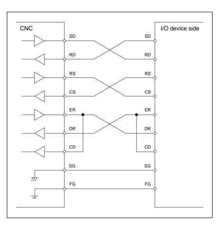
• When the ER signal and the DR signal are not used for a handshake, the following connection is used.
