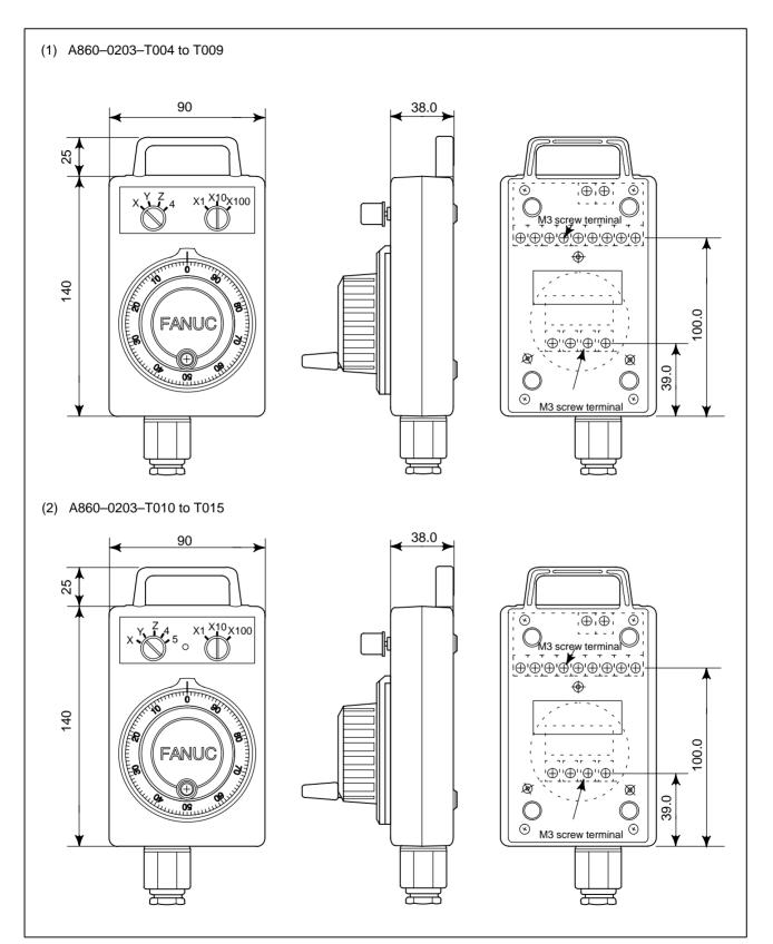
Fig.U19 Pendant type manual pulse generator Specification No. : A860–0203–T004 to T015
