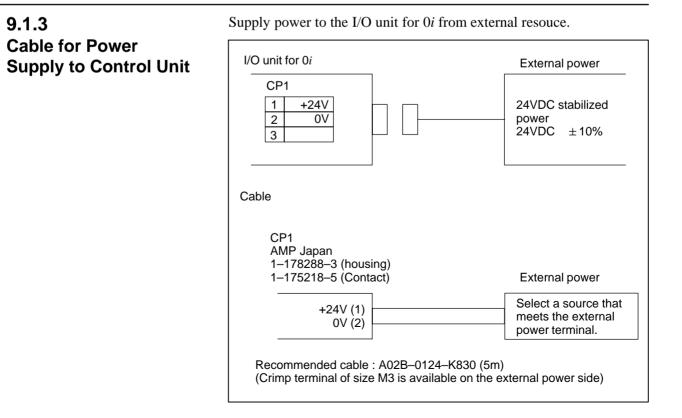
Part of the 24 VDC power input to CP1 can be taken out from CP2 by branching. CP2 should be connected as shown below. In this case, the rating of the external 24 VDC power supplied to CP1 must be the sum of the power consumed within the control unit and that supplied to external equipment via CP2. The maximum capacity of power that can be obtained from a branch is 1.0 A.
