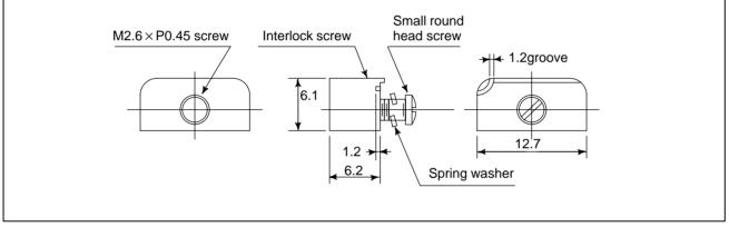
Fig. C8 (b) Locking plate plate for reader/puncher interface connector
