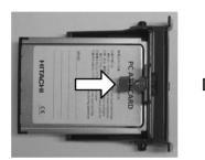
Insert the memory card into the fixing bracket in the direction indicated by the arrow.
