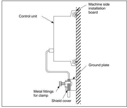
Fig. 3.5.5 (b) Cable clamp (2)
