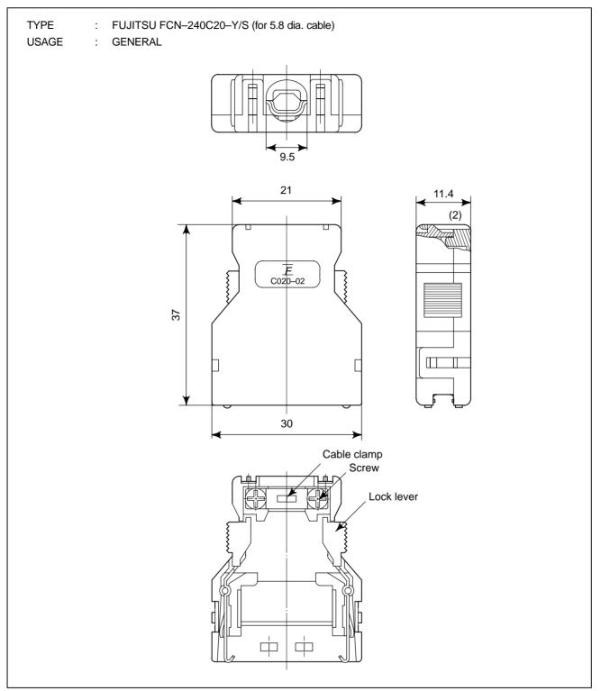
Fig. C2 (c) Connector case (FUJITSU FCN type)
