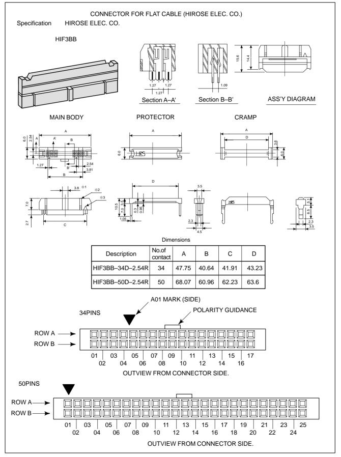
Fig. C6 Connector for HIROSE Flat cable
