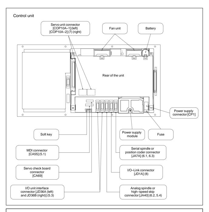
This figure is a rear view of the control unit without option slots.
