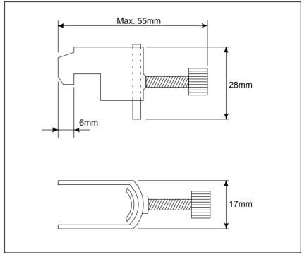
Fig. 3.5.5 (e) Outer drawings of metal fittings for clamp
