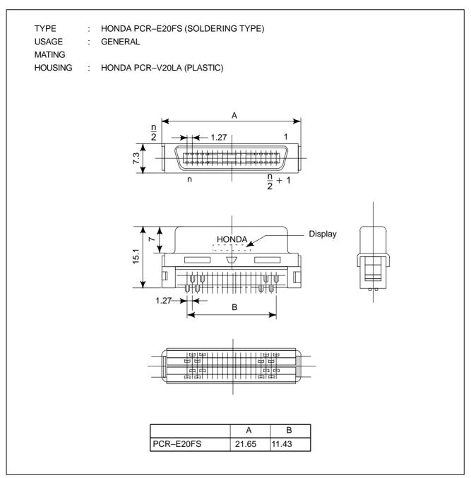
Fig. C1 (a) PCR connector (soldering type)
