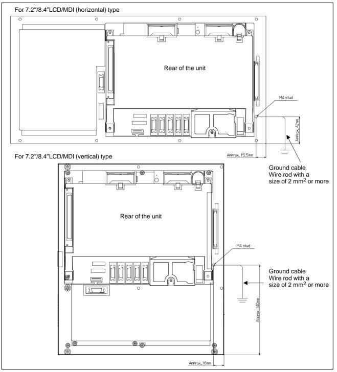
Connect the 0 V line in the control unit to the ground plate of the cabinet via the protective ground terminal (shown in the above figure). For the positions of ground terminals for other units, see the unit outline drawing in the appendix.
