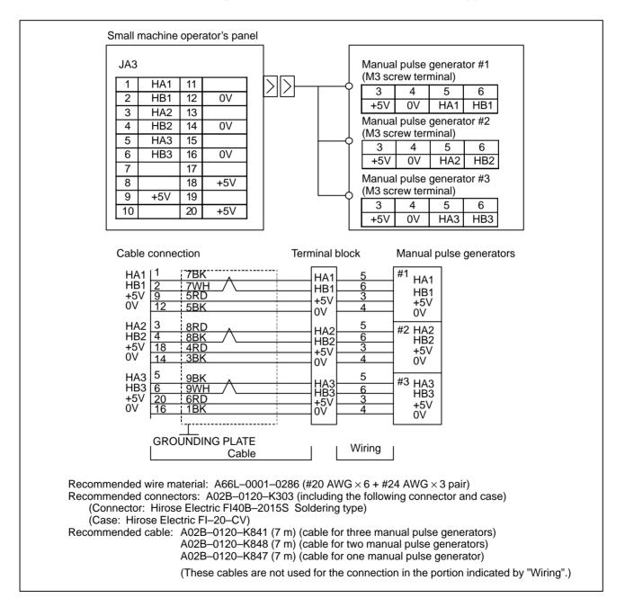
Calculate the maximum allowable length of the cable for the manual pulse generator, with the method described below.
