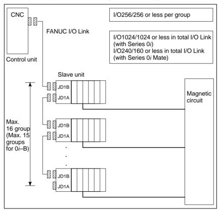
Fig. 8.2 I/O Link connection diagram
