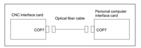
Compatible cables (optical fiber cables, used for interconnections) A66L-6001-0026#L\_
