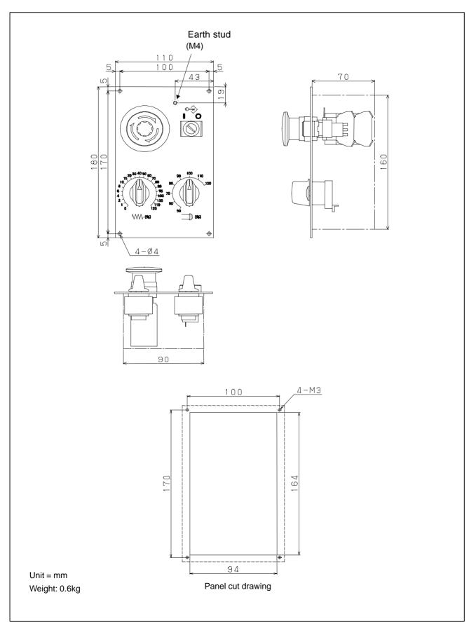
Fig.U27 Machine operator's panel (Sub panel B1) Specification No. : A02B–0236–C235
