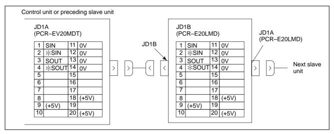
+5 V terminals are for an optical I/O Link adapter. They are not necessary when connecting with a metal cable.
