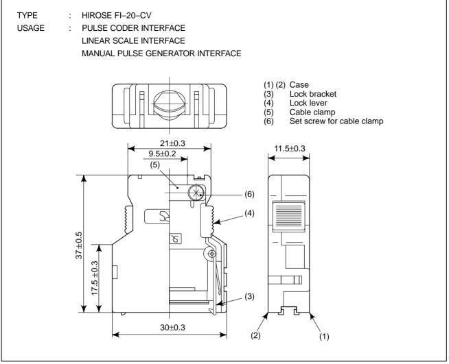
Fig. C2 (b) Connector case (HIROSE FI type)
