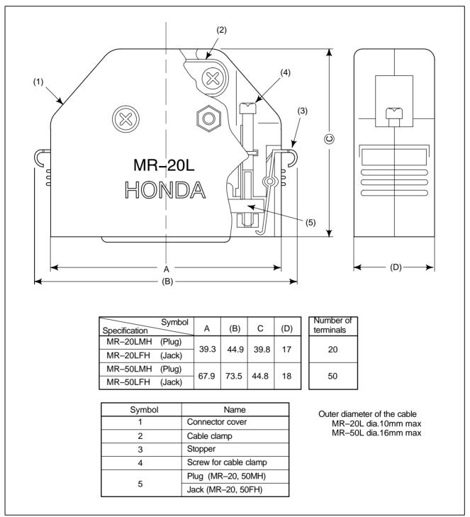
Fig. C4 (a) HONDA connector (case)
