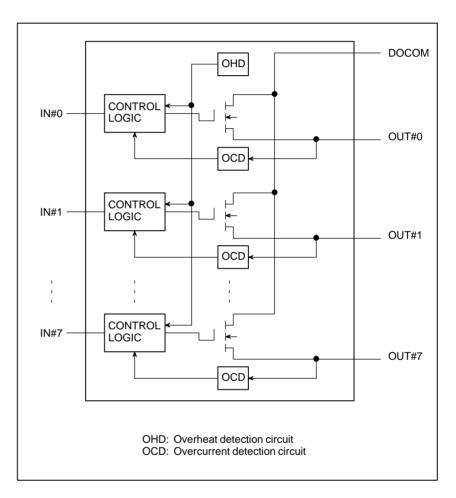
The power for operating this driver element is supplied from DOCOM (24 VDC).
