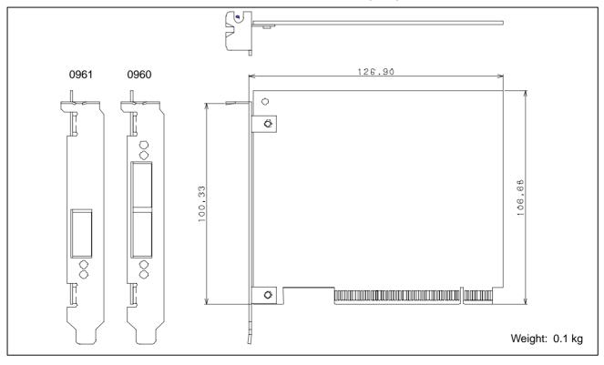
Fig.U16 (b) Interface Board for Personal Computer (PCI bus version) Specification No. : A20B–8001–0960 (2 CH) A20B–8001–0961 (1 CH)
