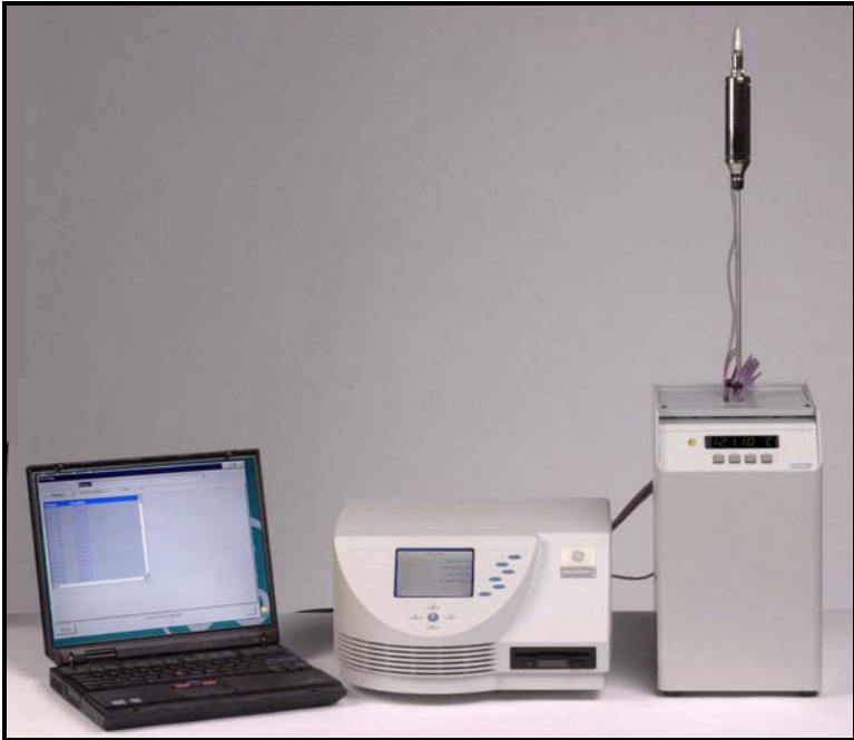
Figure 1-1: Intelligent RTD Probe used for Calibration with GE Kaye High Temperature Reference
