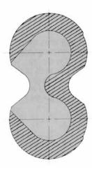
Area of pressure loading shaded (system pressure applied on rear faces of bearing blocks) Area of separating force shaded (sealing surface between bearing surface and gears)
