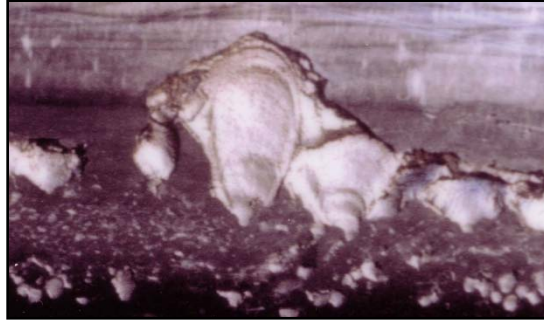
Figure 19. Surface fatigue spalling [36]
