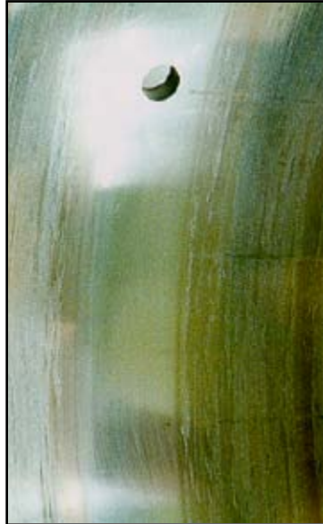
Figure 23. Adhesive wear produced by overheating [33]
