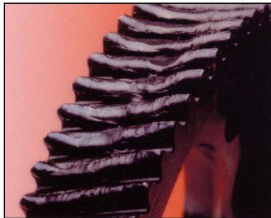
Figure 20. Plastic flow failure [36]
