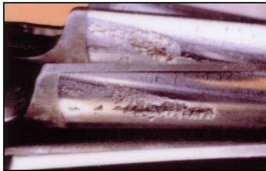
Figure 18. Surface fatigue macropitting [36]
