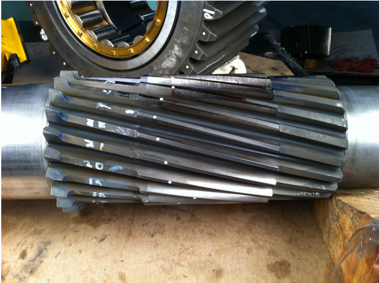
Figure 45. HS pinion scuffing most likely caused by lubricant starvation (Courtesy GEARTECH)
