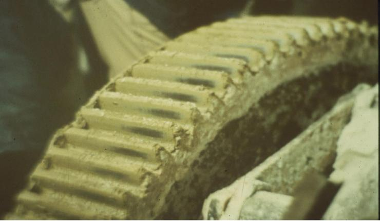
A. The choice is either broken teeth or rapid wearB. Don't forget the two basic metallurgies
