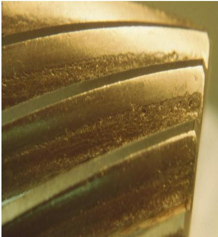
Compressor drive gear after 10 years at 1800 rpm.
