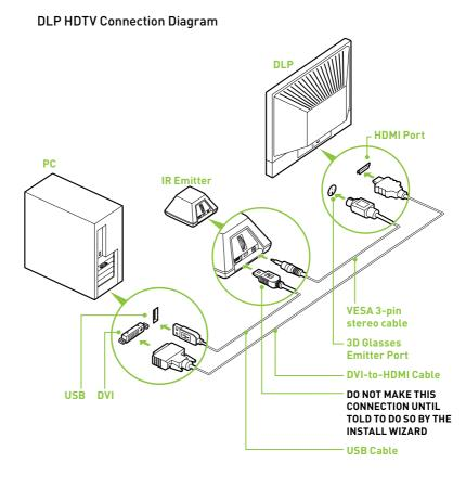
**Note:** Check your DLP's user manual to see if there is a specific HDMI port used to connect a PC to your HDTV. In addition, change the input mode on the TV's menu to be **PC** or **Computer** to ensure the TV can process the video signal correctly.
