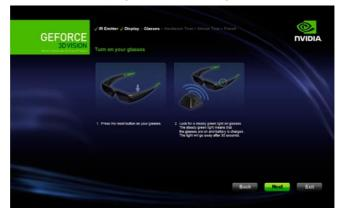
Press the **ON** button on your glasses. You should see a steady green light on the glasses. The green light means that the glasses are on and the battery is charged with up to 40 hours of gaming time (on a full charge). The light goes out after approximately 30 seconds.
