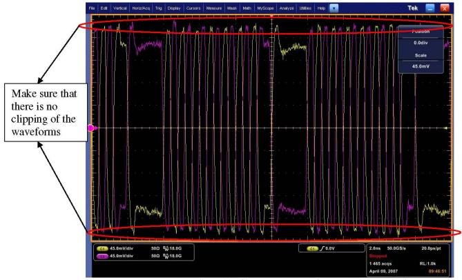
Figure 11. Single Ended Data full scale without clipping
