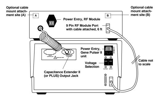
Fig. 3. Red/black leads and the 9 pin cable of the RF module (back panel) connected to the appropriate output jacks and port on the back panel of the Gene Pulser II unit.
