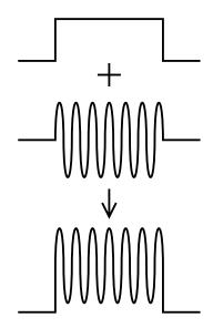
Fig. 1. The FlexWare technology of the Gene Pulser II RF module delivers the unique combination of a pulse of radio-frequency (RF) field and a DC pulse with the same pulse width for improved transformation.
