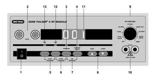
Fig. 5. The control panel of the RF module. Front panel identification of switches and keypads for the RF module. Note that the keypad(s) are active when the light(s) above them are illuminated.
