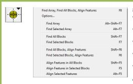
Align Blocks— Gives you multiple options for finding array, finding blocks, and aligning features within those blocks. The menu lists functions in order of most to least automated from top to bottom. Selecting the Options... item from this menu directs you to the Options dialog — Alignment tab described in previous slides.
