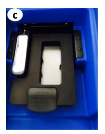
NOTE: The scanner fires the laser from below, so sample surface must be facing down in the holder.
