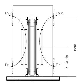
Airflow necessary to dissipate the total transformer losses inside the enclosure is defined by the following formula:
