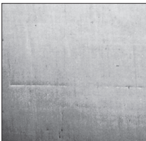
Scratch remains due to overload.
