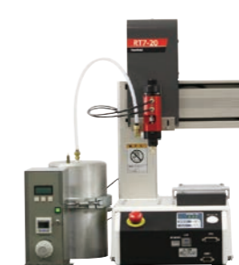
Tank for 1-kg can (PT-01) Needle type dispense valve (HPNV-50) Pressure controller (coater S4) Desktop 3-axis robot (RT7 Series)
