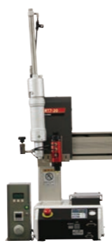
Cartridge-type tank (LVCT-AC) Diaphragm type automatic valve Controller for pressure (coater S4) Desktop 3-axis robot (RT7-20)
