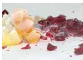
Material embrittled with liquid nitrogen
