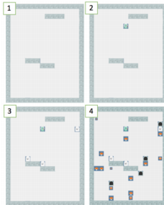
Figure 3 - Step-by-step process the constructive generator takes in building a level [6].
