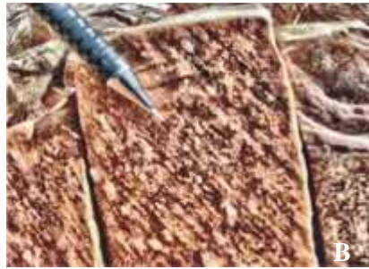
Figure 5.9. (A) Strike-slip lineation ( 0-15^\circ ), (B) Oblique-slip lineation ( 15-45^\circ ), (C) Normal-slip lineation ( >45^\circ ).
