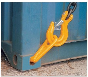
Figure 2: Typical Side Lifting Lugs, showing top and bottom arrangements.
