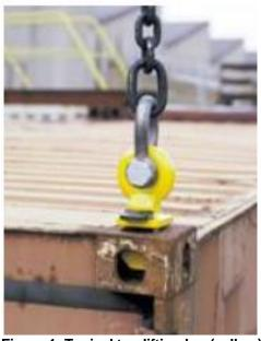
Figure 1: Typical top lifting lug (yellow)
